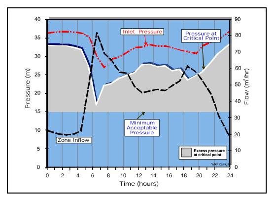
Figure 1.10: Typical zone with no pressure control
