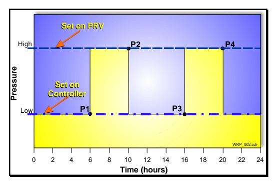
Figure 1.4: Typical 4-point time modulated pressure profile
