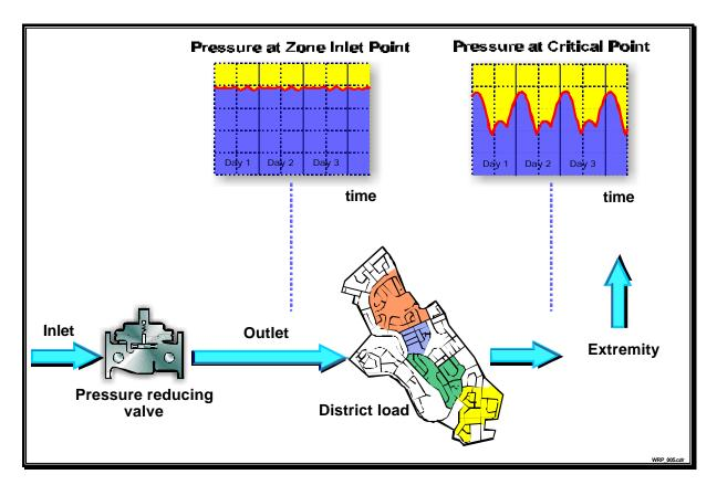
Figure 1.3: Pressure control using conventional PRV
