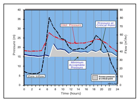
Figure 1.13: Typical zone with flow-modulated pressure control
