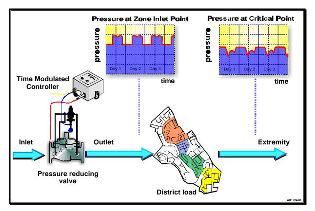
Figure 1.6: Pressure control using a time-modulated PRV controller
