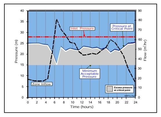
Figure 1.11: Typical zone with fixed-outlet pressure control
