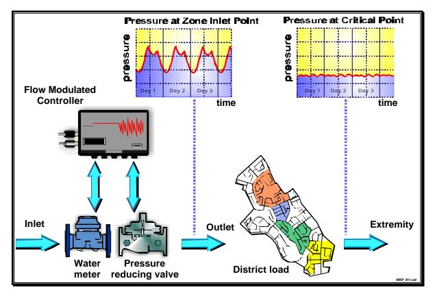
Figure 1.8: Pressure control using a flow-modulated PRV controller
