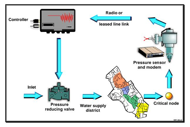
Figure 1.9: Pressure control using a telemetry linked flow-modulated PRV controller
