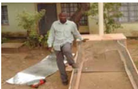
Direct Mode-Solar Sludge Drier
