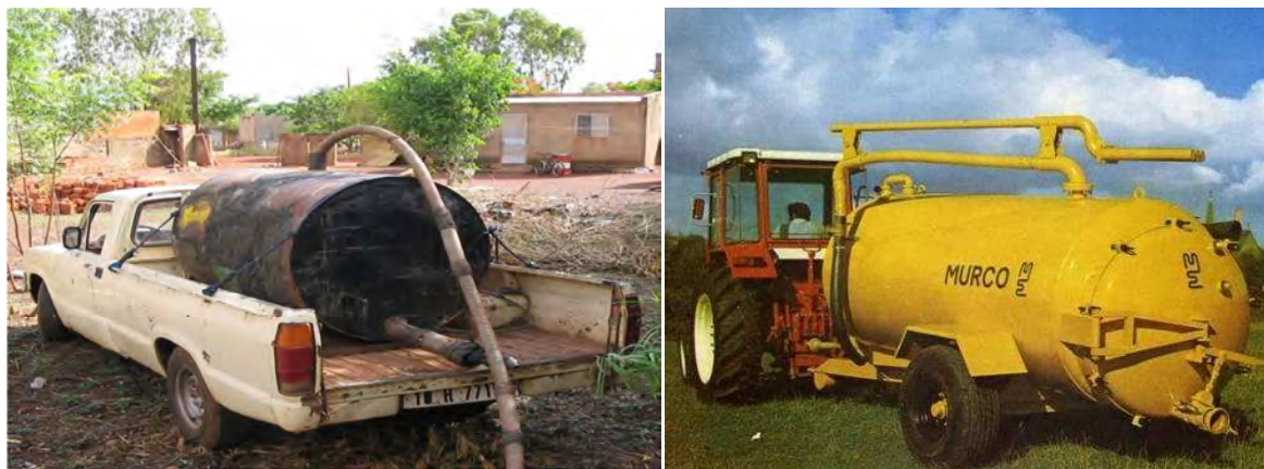
Figure 4.15 Tankers carried on a truck bed (left, EAWAG) and pulled by a tractor (right, Manus Coffey)
