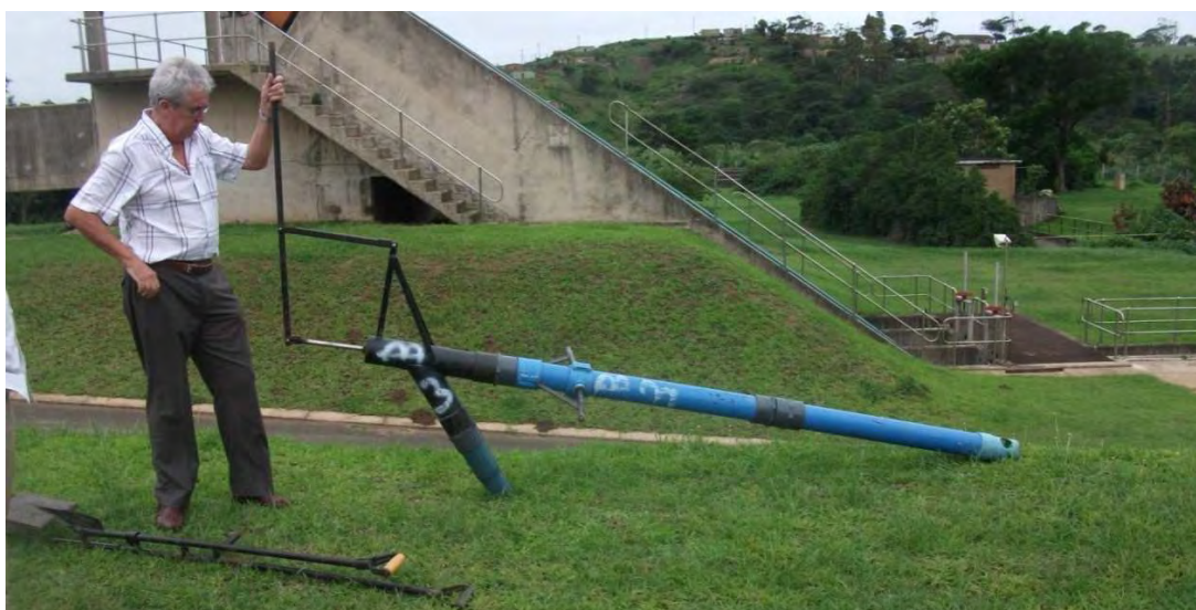
Figure 4.11 The Modified Gulper, with lever action added
