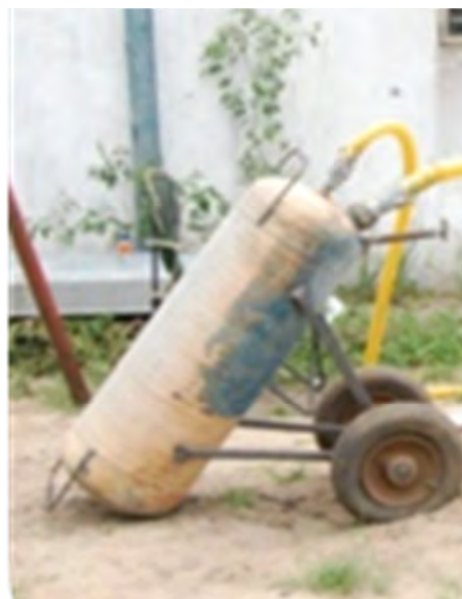
Figure 4.33 Gas canister used as a pressure vessel for the NanoVac
