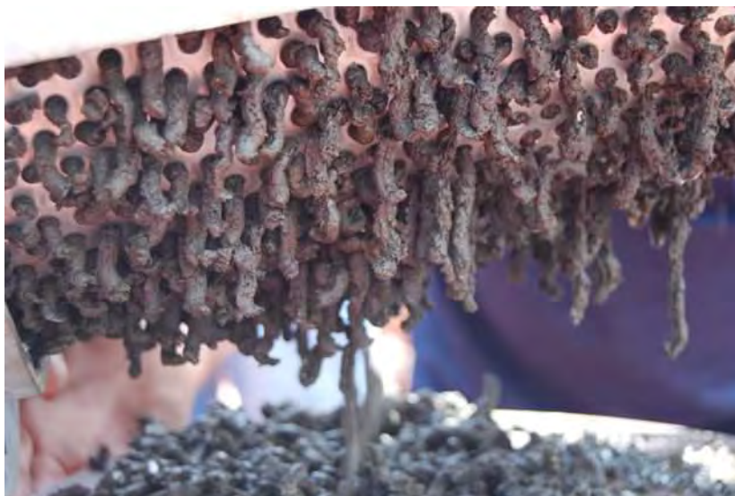
Figure 6.22 Sludge being extruded through a screen prior to heat treatment
