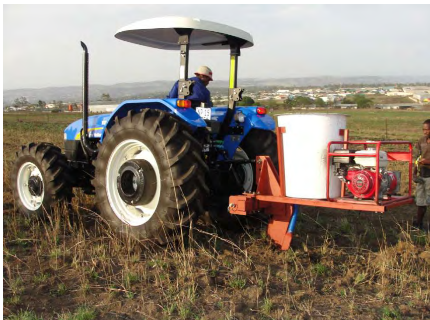
Figure 6.21 Field testing the sludge injector
