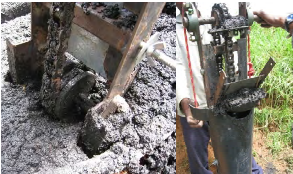
Figure 4.29 Prototype of Gobbler with single chain and sprung scraper
