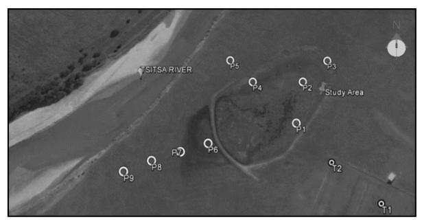
Figure 3-13: Location of piezometers and sampling sites of the first instrumented wetland.
