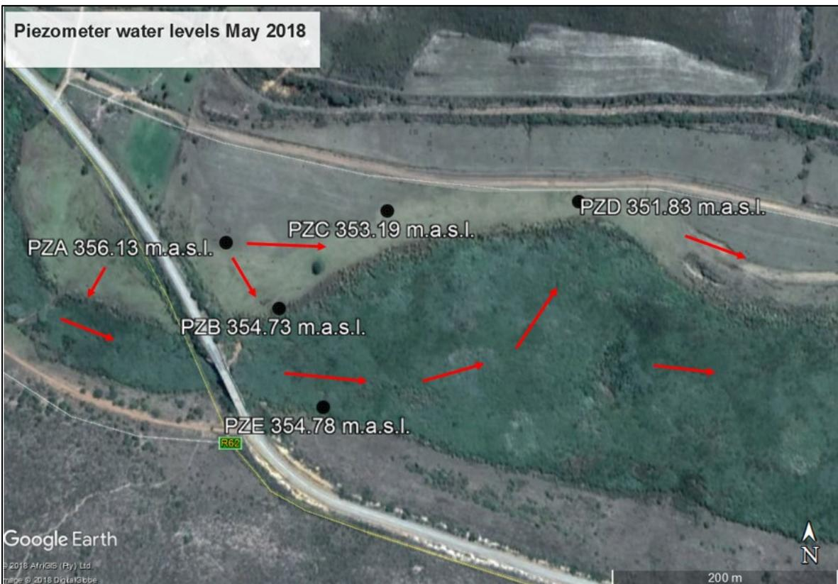
Figure 35: Proposed subsurface flow directions at the Kompanjiesdrif wetland with water levels measured in May 2018
