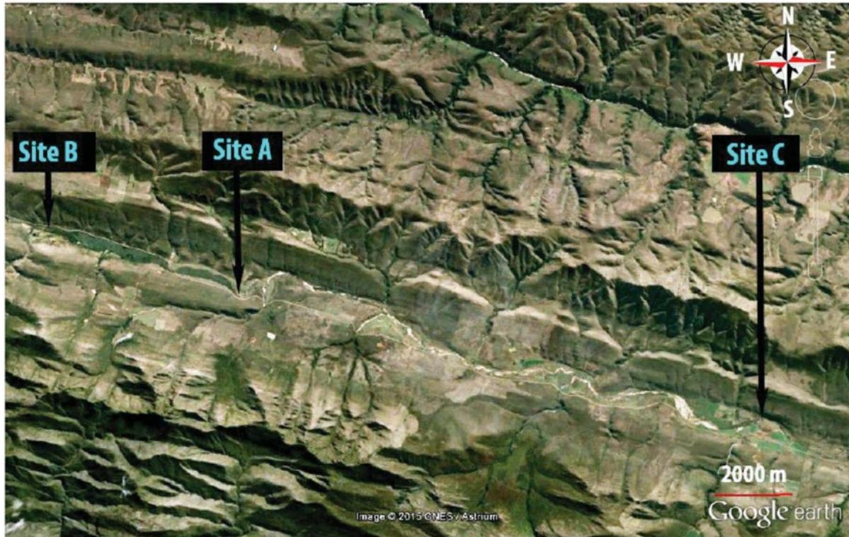
Figure 56: Sites of subsurface water level measurement through piezometers installed adjacent to erosion-control structures (at Site A) and potential structures (Site B and C)
