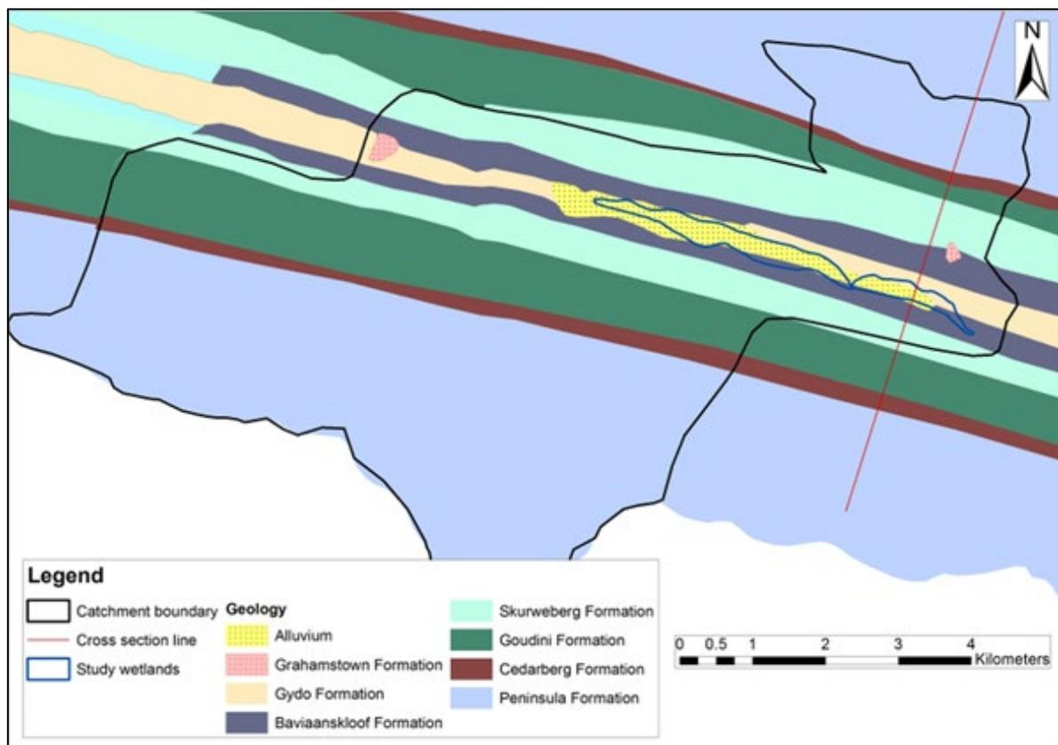
Figure 11: The geology of the study catchment based on the 1:250 000 geological map (Toerien, 1986) with the location of the cross section (illustrated in Figure 12) indicated by the red line
