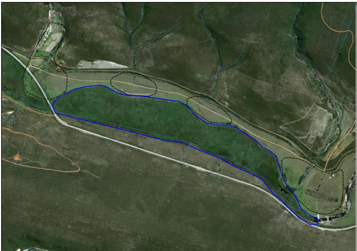
*Figure 10: Alluvial fans (stippled black line) impinging on the Kompanjiesdrif wetland, curbing the extent of the wetland*
