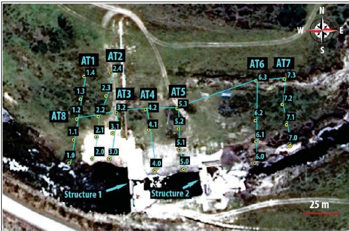
Figure 57: The locations of transects at Site A. Transect AT1 is along the non-eroded reach and AT6 is along the eroded reach downstream of the erosion-control structures
