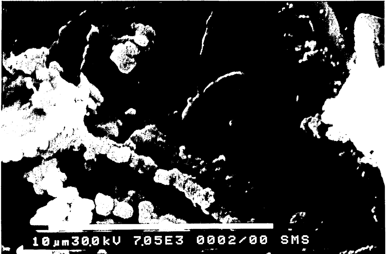
FIGURE 11 SCANNING ELECTRON MICROGRAPH SHOWING ATTACHED BACTERIA ON THE SURFACE OF A MILD STEEL SAMPLE
