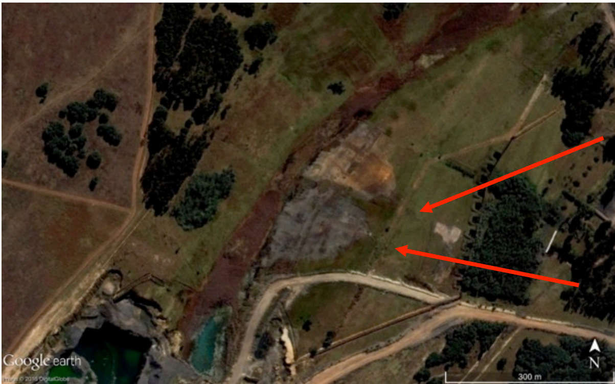
Figure 60 Acid water outflow zone (with visible plume) through boreholes (red arrows) that “punctured” an underground disposal facility
