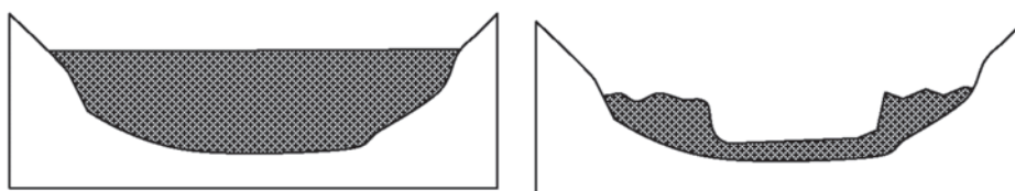
Figure 21: Schematic cross-section through the Krugersland/Companjesdrift peat basin, showing the current situation (a) compared with an incised situation (b). Given the present state of the channel at the distal end of the basin and the drop in level (2-3m to bedrock) that has occurred since that year, the threat to the basin has increased considerably.
