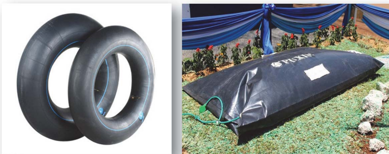
Plate 4-8: Tractor tyre tubes (left) or specifically designed biogas storage bags (right) can be used for gas storage (source: Linea Tyre n.d.; Takamoto Biogas 2011)
