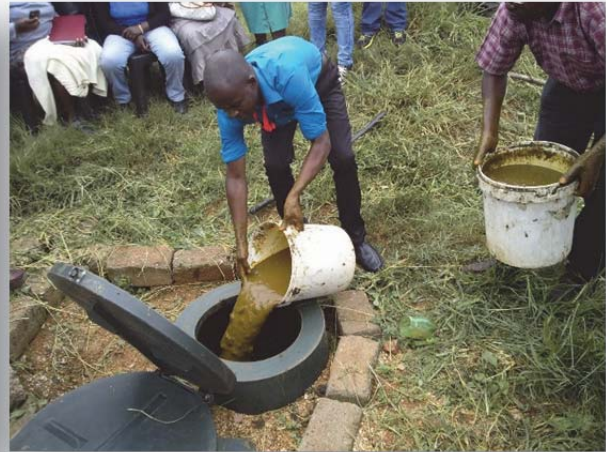
Plate 4-15: The manure-water mixture is mixed by hand or using an implement (left), and then poured into the digester once thoroughly mixed (right)
