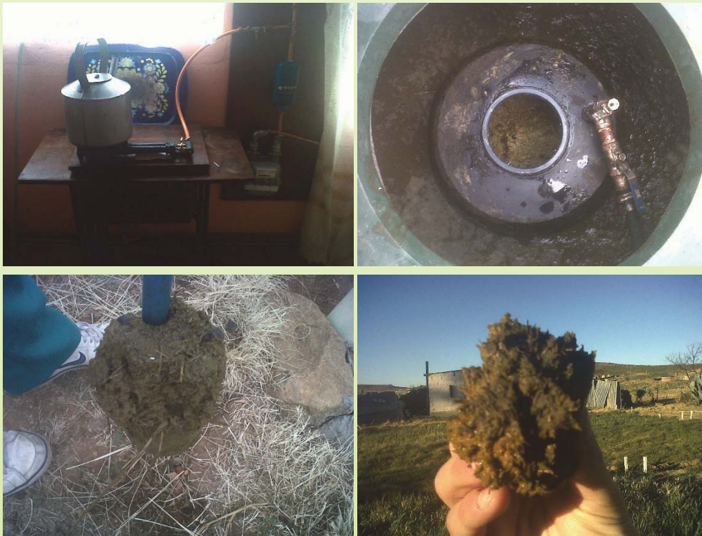
Plate 4-24: Clockwise from top left: (a) High gas pressure, minimal gas, (b) opened gas chamber, (c) solid mass of ligneous material, and (d) light fluffy consistency of the ligneous material
