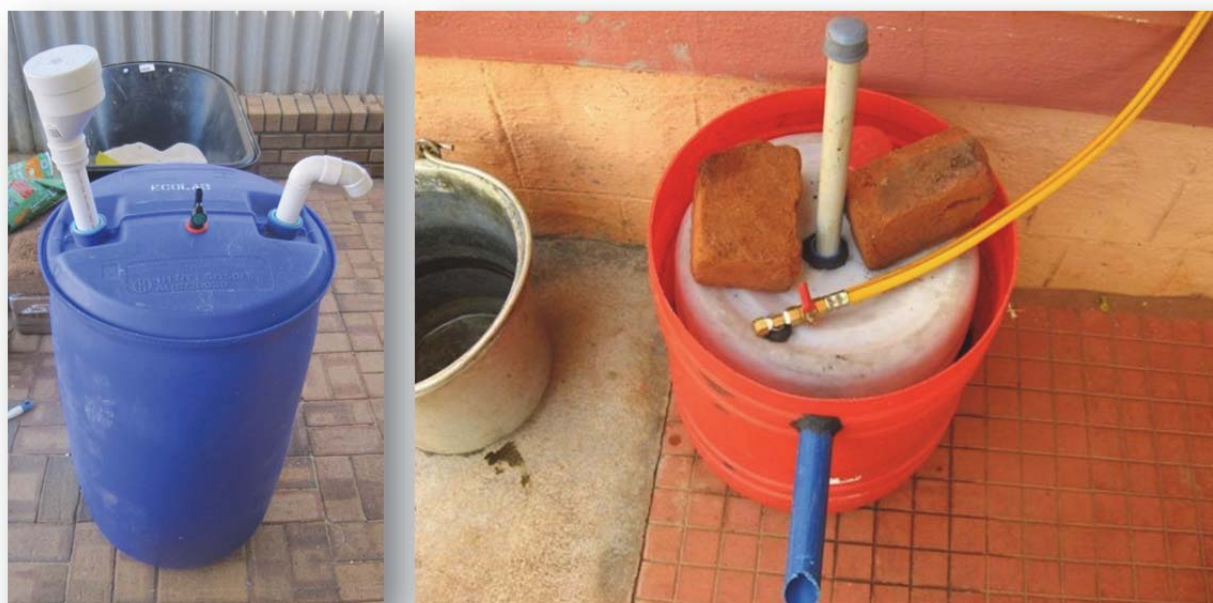
Plate 4-7: Various simple tank digesters (source: Burton 2014; Antoniraj 2015)
