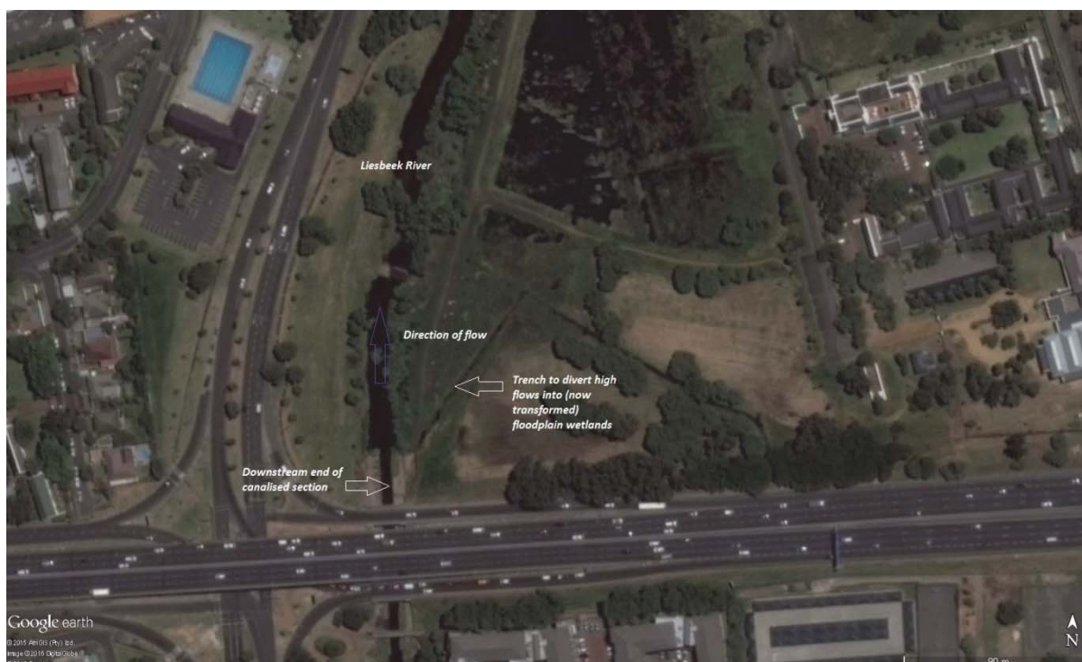
Figure 10.19: Floodplain reconnection between the channelised / canalised Liesbeek River and adjacent off-channel depressional wetland areas. Rehabilitation works undertaken by Friends of the Black and the Liesbeek River
