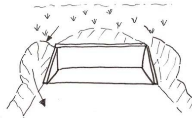
4. 'Weir' outflanked by erosion after flood because there was no means of guiding the water to the spillway
