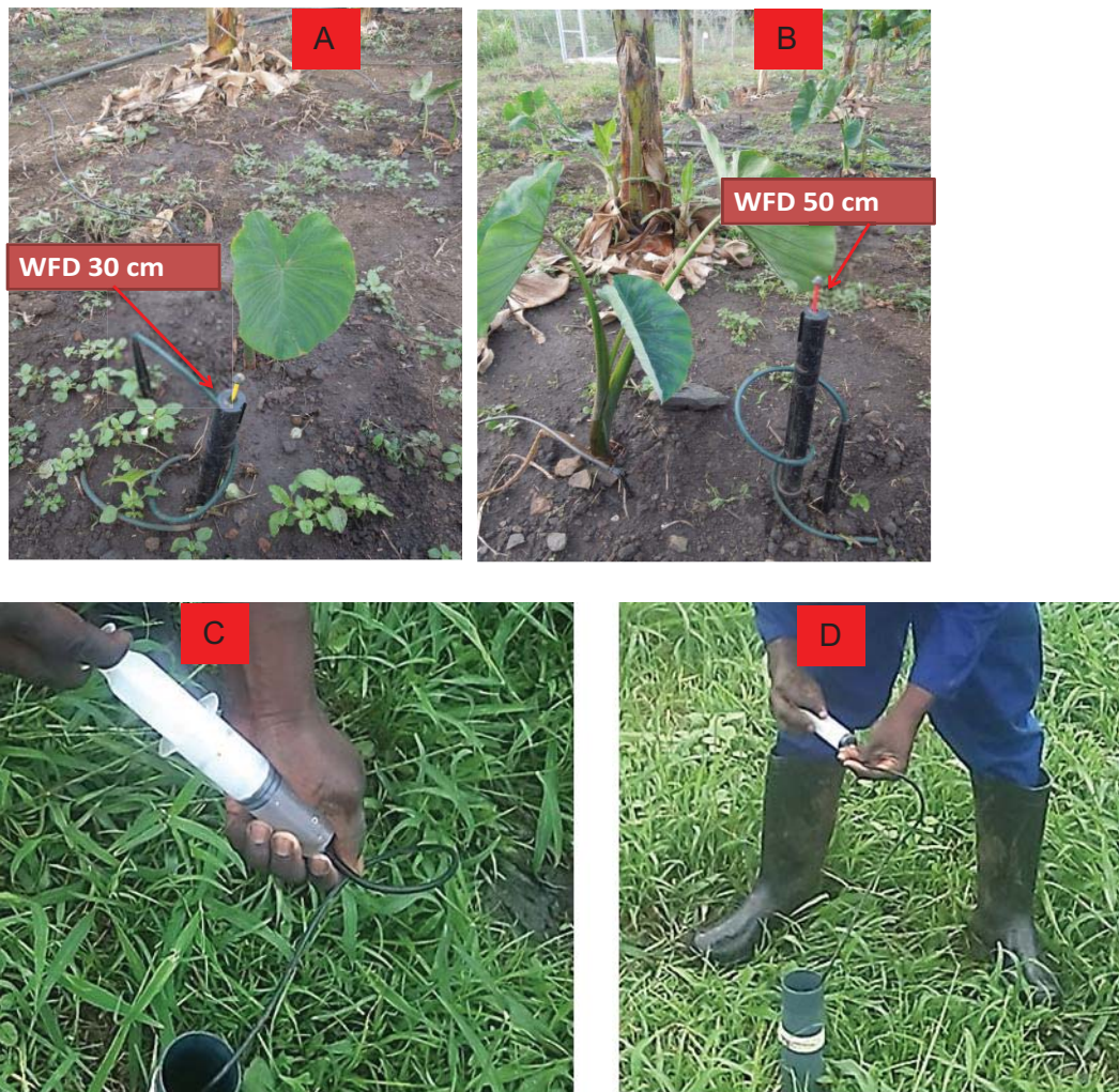
Figure 3.10 Wetting front detectors at (A) 0.3 m and (B) 0.5 m; collection of leachates from the piezometers at 1 m to collect leachates from (C) within and (D) below the root zone
