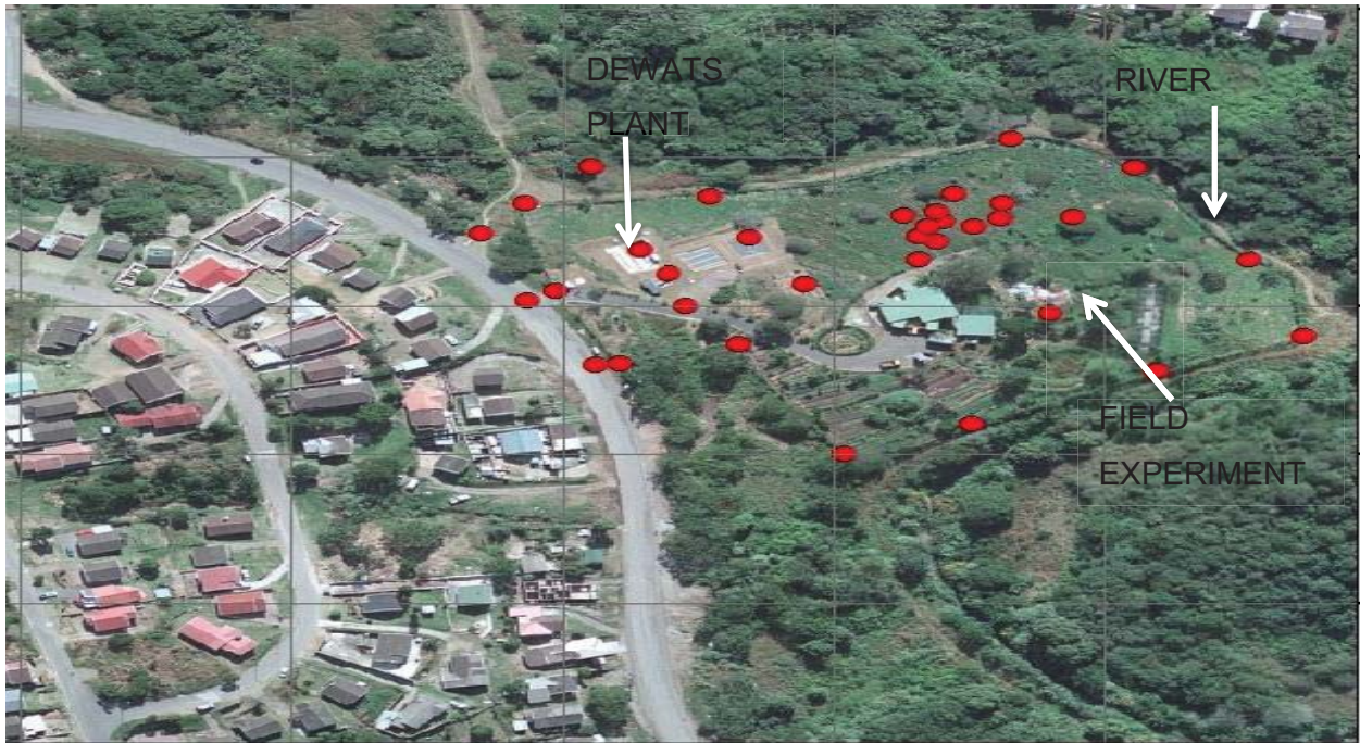
Figure 3.1 An aerial view of Newlands-Mashu site showing the DEWATS (ABR) plant, the experimental site, physical features (river) and some of the contributing houses. The red dots are GPS points
