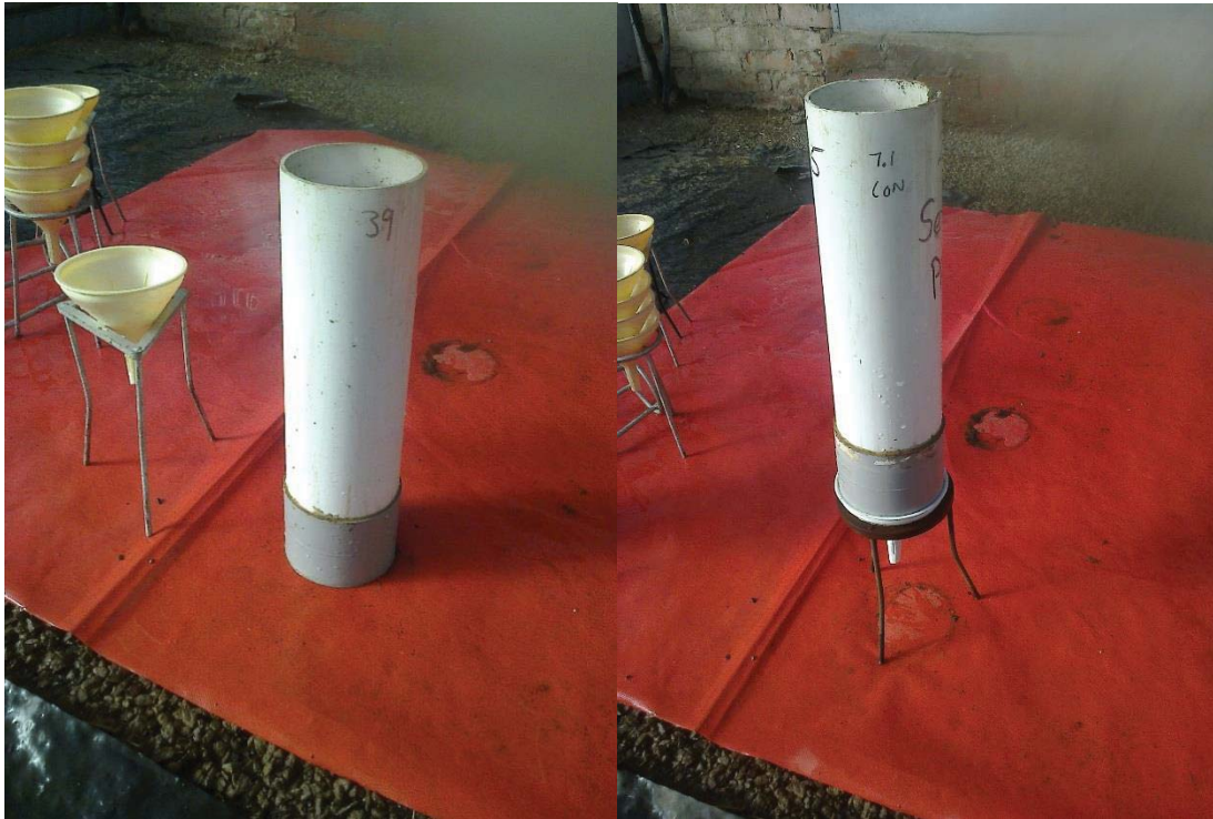
Figure 4.15 Experimental unit for the soil column experiment
