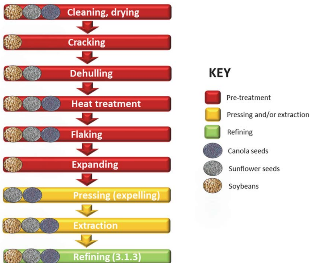
Figure 8: Flow diagram showing the different typical industrial-scale pre-treatment, pressing and extraction steps for Canola seed, sunflower seed and soybean oil production
