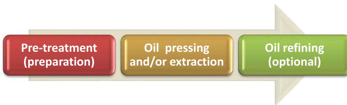
Figure 6: Edible oil production can be divided into 3 major processes that differ according to the starting material and personal choice of the manufacturer
