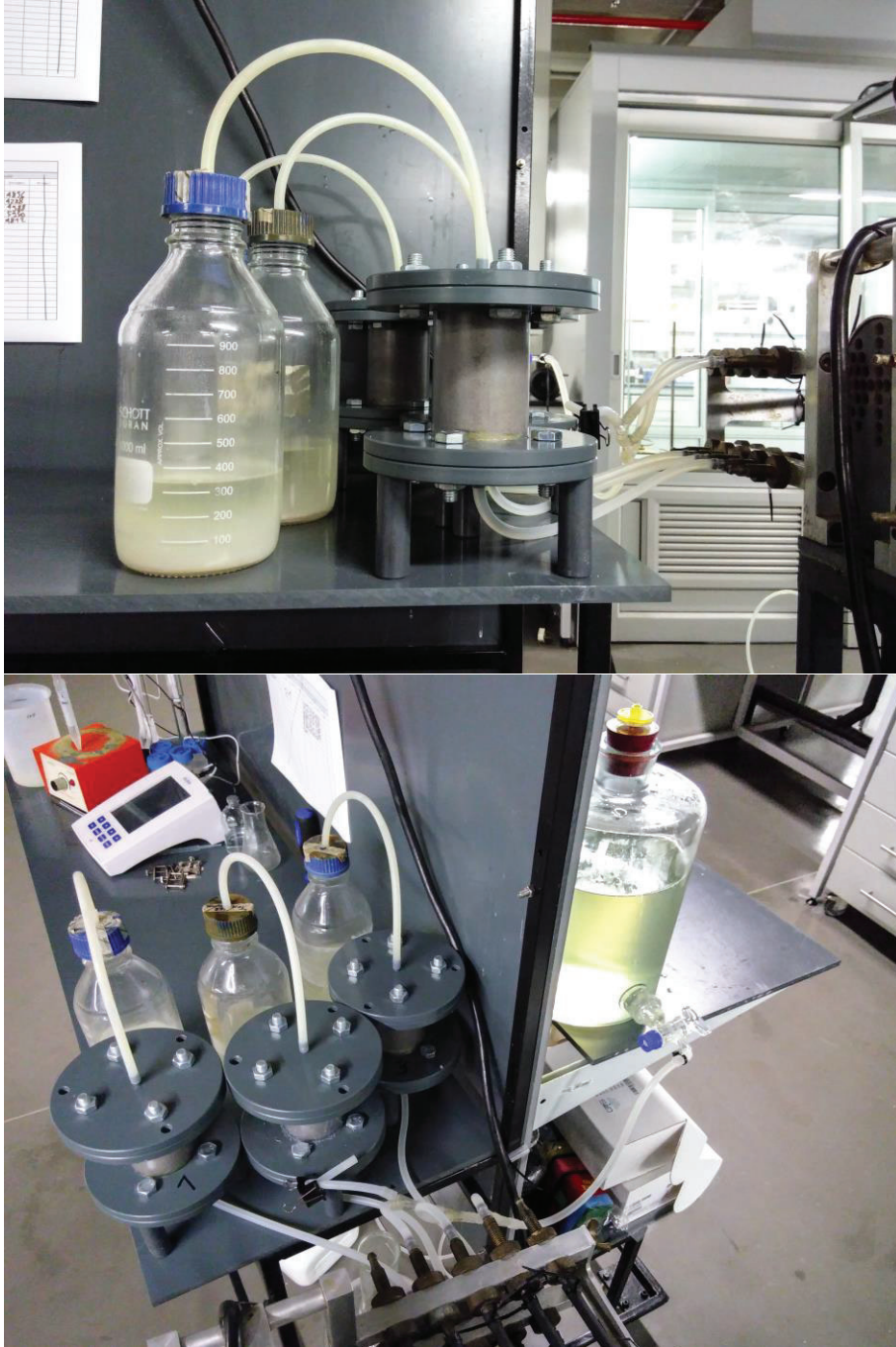
Figure D. 1: The reactor setup used in Experiment 1 & 2. Top: Cementation media is injected from the bottom to the top and the effluent is collected in 1 L bottles. The approximate setting of the flow rate could be monitored by the collected volume of effluent. Samples were manually captured in separate glassware. Bottom: The peristaltic pump (bottom, center) was controlled by a timer switch. Each reactor had its own, independent tubing. The influent container on the right has a volume of 5 L and the air inlet on top was equipped with a 0.45 \mu m filter.
