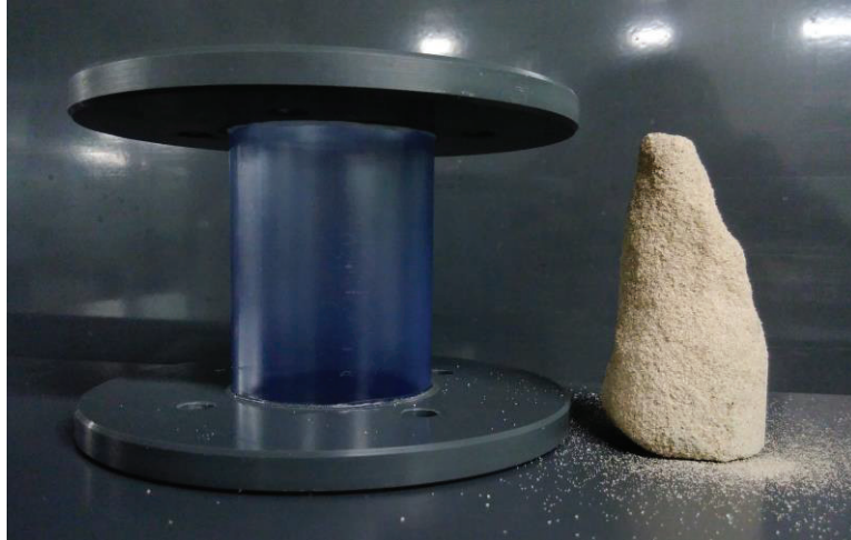
Figure D.2: The solidified part recovered from one reactor in experiment 2. The surrounding sand did not show any sign of solidification. This indicates the effect of a preferential flow path during inoculation.
