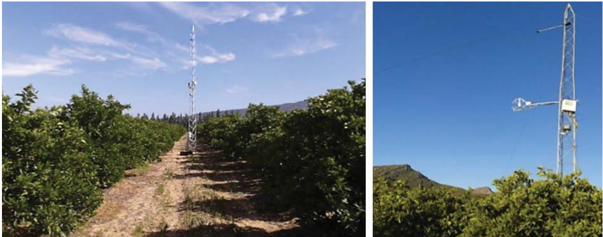
Figure 3.17 Lattice mast in the ‘Washington’ navels orchard showing position of eddy covariance sensors
