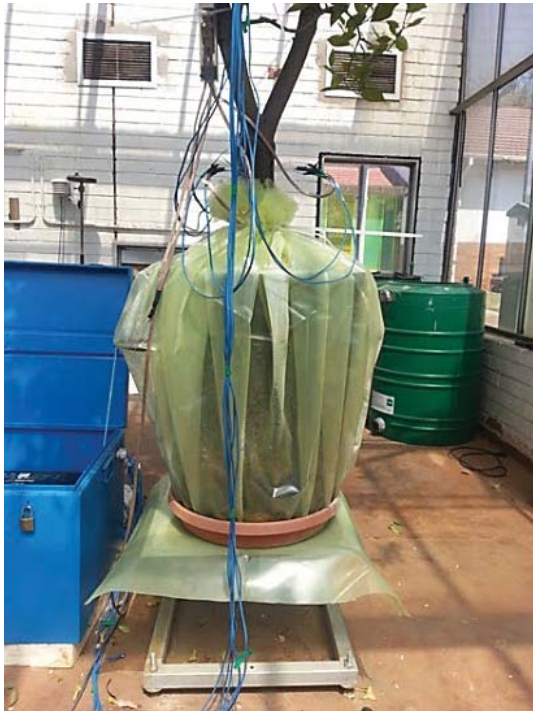
Figure 3.10 Placement of the 'Midnight' Valencia trees on the weighing lysimeters and probe installation. Note the plastic covering to eliminate evaporation and drainage from the pots
