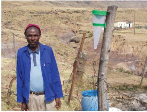
(a) A homestead rain gauge in Sinxaku. Daily rainfall is collected in a notebook.
