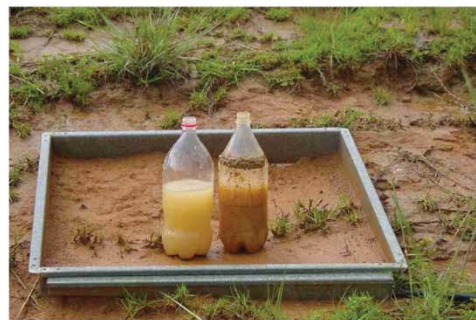
(e) Runoff plots for comparing response of different areas. Runoff and sediment lost from the plots is collected downslope in a container connected to the lower end of the plot by a plastic pipe. A 20 litre container is recommended where rainfall is heavy.
