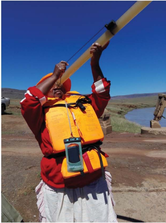
Using a clarity tube to estimate turbidity
