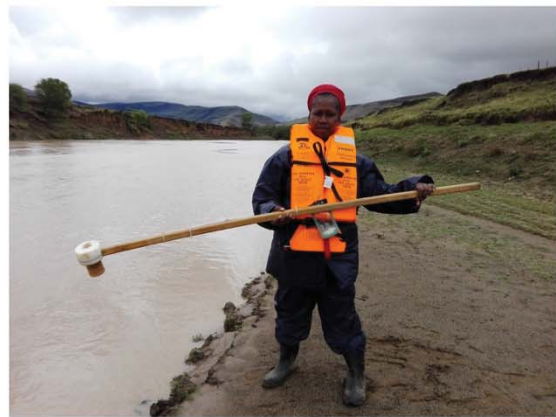
The water sampler with water bottle full of a sample
