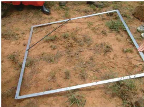
(b) A quadrat used to measure basal cover of vegetation. By dividing the quadrat into 100 square (10x10) the percentage of ground cover by rooted vegetation can be estimated. The quadrat should be placed at the same point for monitoring changes through time. The location of opposite corners of the quadrat should be marked permanently on the ground.
