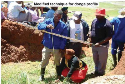
(c) Profiling a donga. Erosion or deposition on a gully floor and changes to gully width can be monitored by profiling a transect between two fixed points. Metal stakes are used to locate the ends of transect. The depth to the gully floor is measured at equal intervals across a stiff wire stretched between the stakes.
