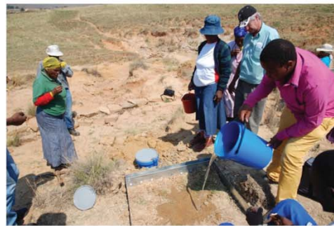
(d) Splash board and graph of data collected by the community. The board measures the intensity of erosion by raindrop impact. The height to which soil particles are splashed onto the board is measured and recorded.
