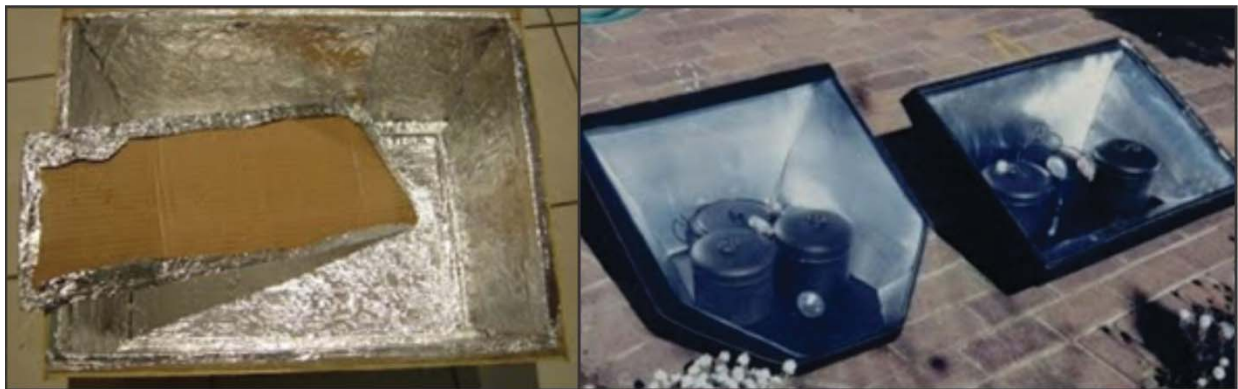
Plate 4.2: A homemade solar cook box (left), and a bought Sunstove solar oven (right)
