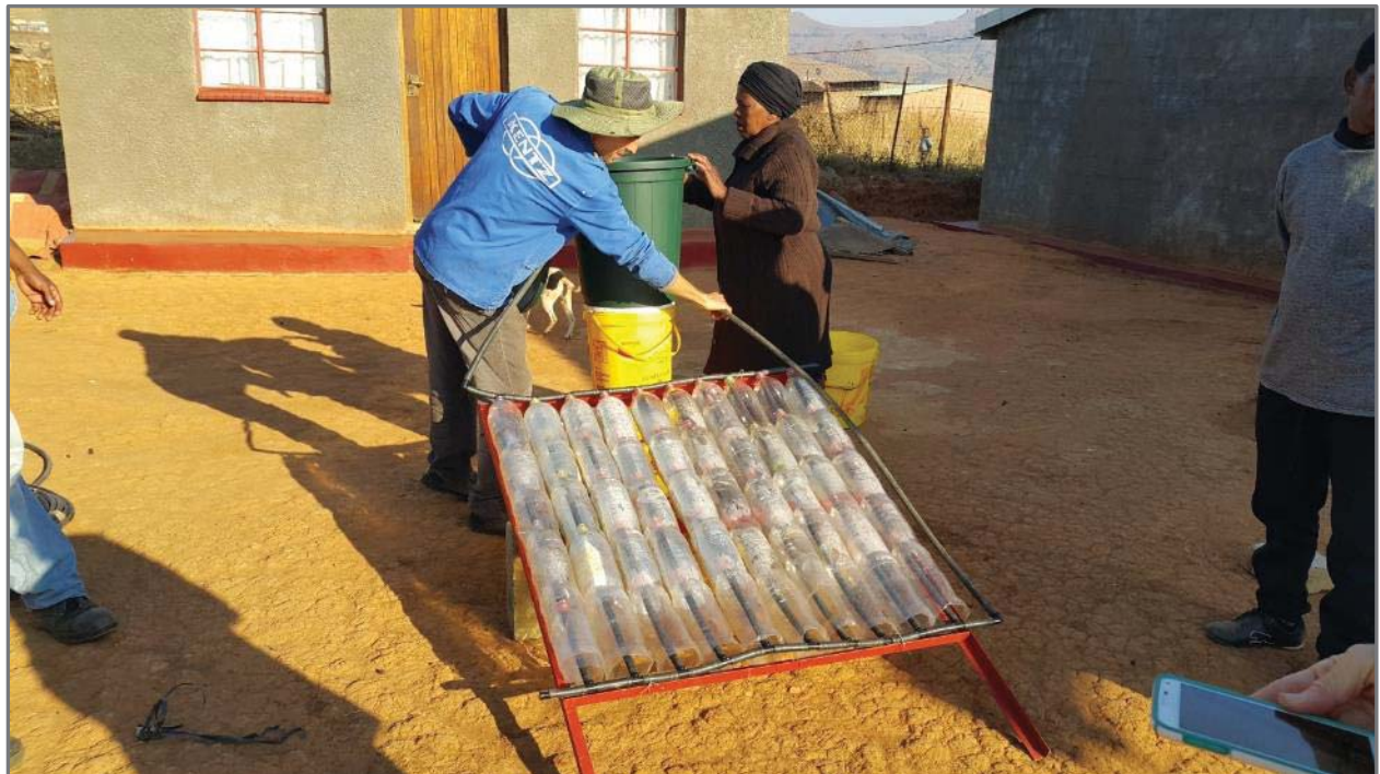
Plate 5.1: A solar geyser made by Mr Tony Lopes and the Mahlabathini Community Research Group.
