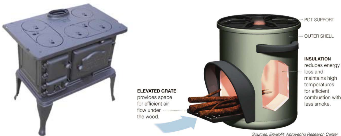
Figure 3.14: An externally vented cooking stove (left) and improved cooking stove (right) (source from left: Ndebele stoves 31 ; Bioenergylists 32 )
