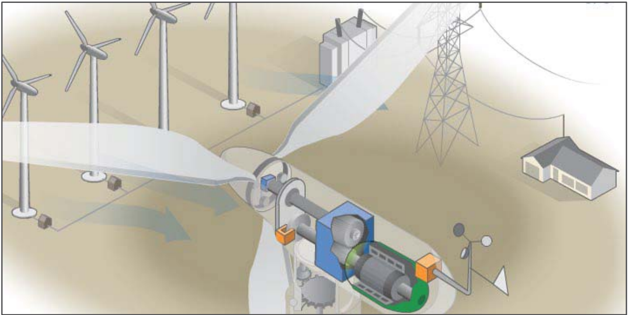
Figure 3.10: Inner workings of a wind turbine (source: U.S. Dept. of Energy 26 )
