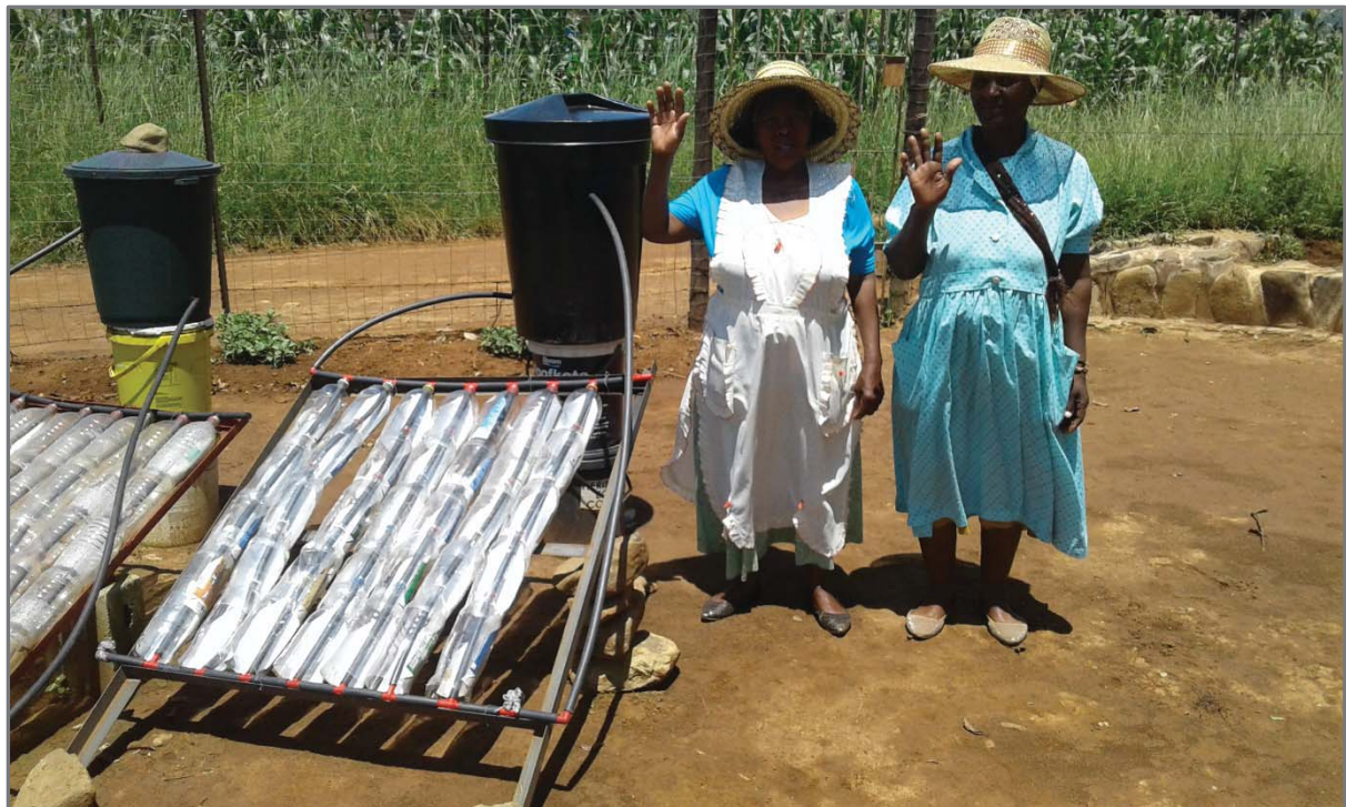
Plate 5.9: Two of the solar geyser production team with the solar geyser that was commissioned by the research team
