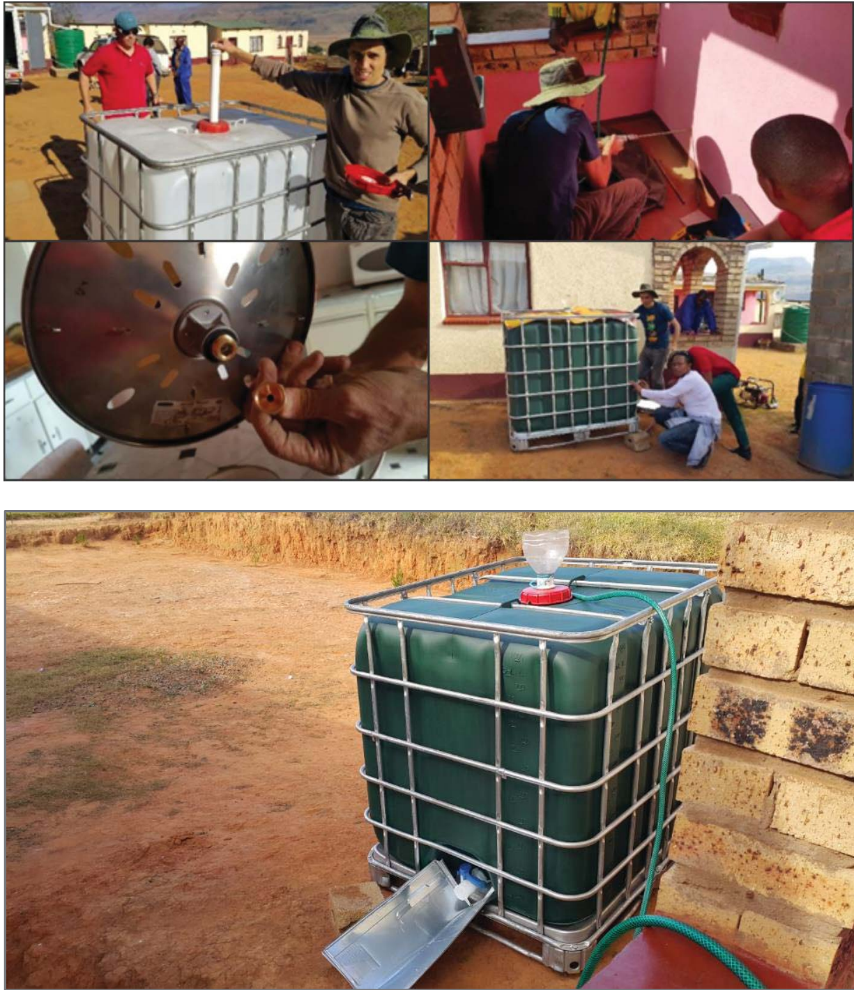
Plate 5.8: A low-tech biodigester manufacturing at Mahlabathini village during a WRC K5/2423 training workshop.
