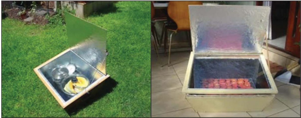
Plate 5.2: 'Low-tech' solar ovens made from plyboard and aluminium sheeting (Lopes, 2016).
