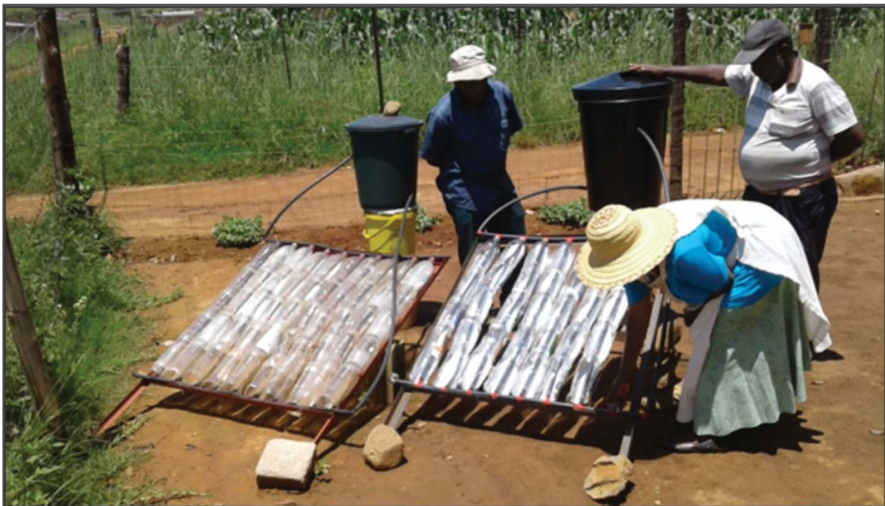
Plate 4.4: Community members inspecting two low-tech solar geysers, one made during the training day (left), and the other made by the community (right)
