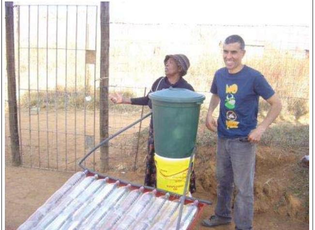
Precious at Okhombe Drakensberg with 10 column geyser and 50 litre container.
