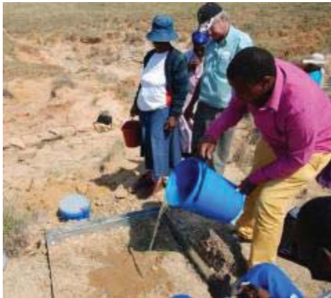
Figure IV-2: Adapted runoff plots with 20 litre collection container
