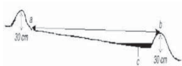
Figure C.3.1-7: Earth bunds – Determining distance between soil bunds
