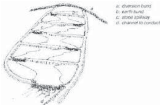
Figure C.3.1-6: Earth bunds – System of earth bunds with stone spillways
