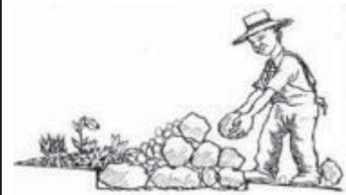
Figure C.3.1-5: Stone bunds – Maintain by filling gaps and tunnels small stone
