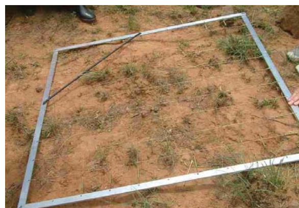
Figure IV-6: Quadrat used to measure basal cover of vegetation
