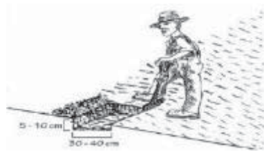
Figure C.3.1-2: Stone bunds – Dig shallow trench along contour line
