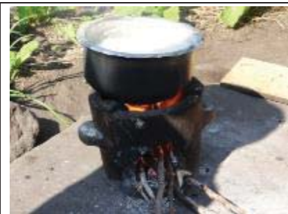
Figure E.5.1-5: Energy Efficient Stove (S. Braid)
