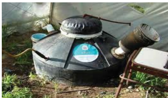
Figure E.5.8-3: Biogas digester c
