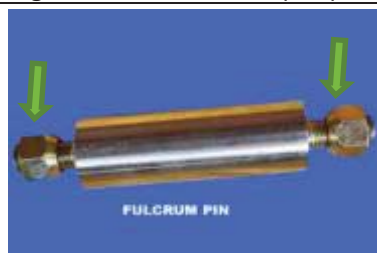
Figure E.3.2-5: Fulcrum Pin Nuts – Check that these nuts are tight. (Source: Joissam Ghana Ltd. 2015)
