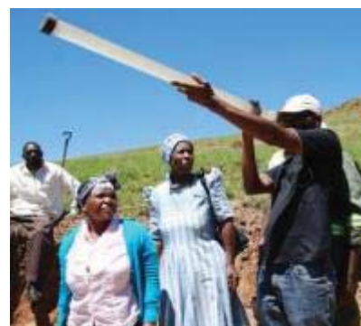
Figure IV-7: Themba Khumalo using a clarity meter to assess water quality
