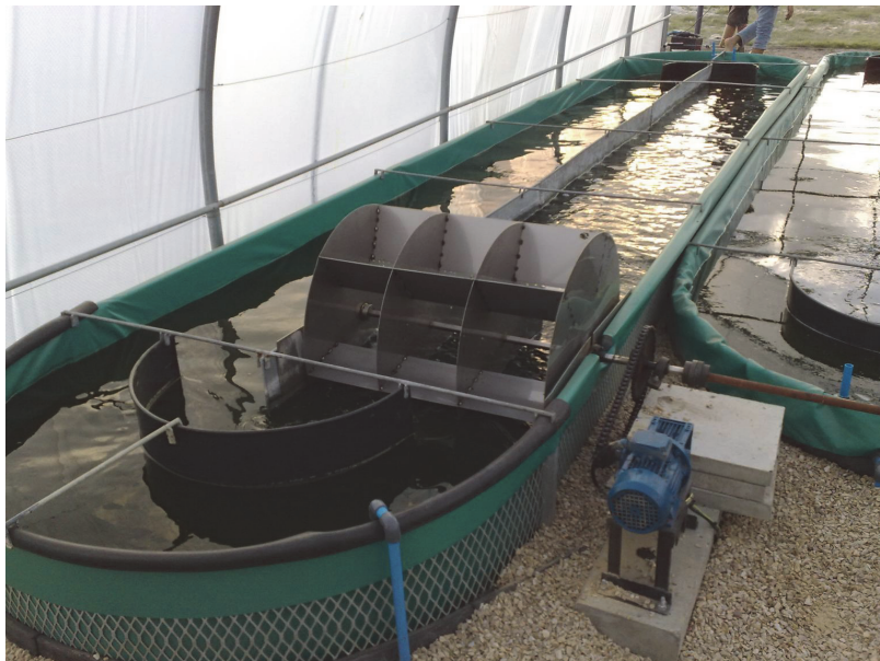
Figure 2.6 High rate algal ponds (HRAP) with a motor operated paddlewheel (Photo: Rory Scheepers).
