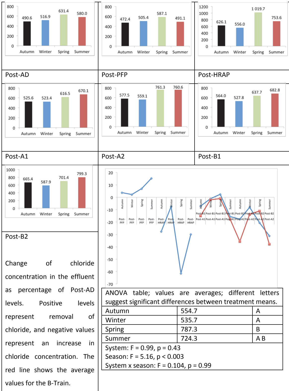
Figure 1.7 Change of chloride concentration (mg/L) in the effluent as percentage of Post-AD levels.
