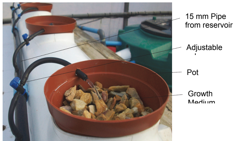
Figure 2.16 The hydroponic system used for all tomato growth trials. Each system included five pot plants with a tomato plant in each (Photo: Sean Power).
