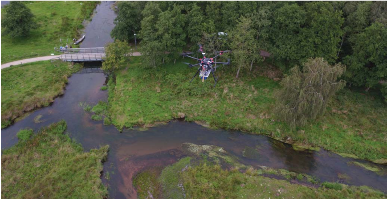
The Riverscapes project, conducted by a consortium led by the Technical University of Denmark (DTU), is developing a drone-based monitoring solution that delivers hydrometric and ecological data to inform catchment-scale risk assessment, channel maintenance and climate change adaption
