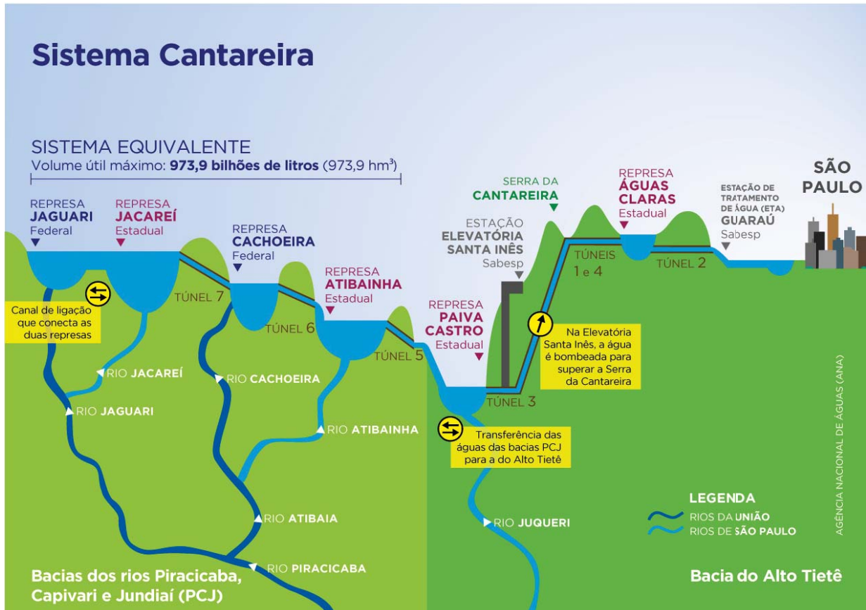
Hydraulic scheme of the Cantareira water supply system
