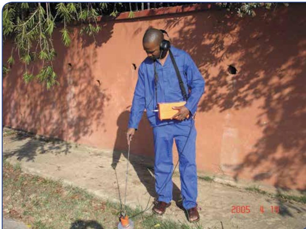
Figure 4: Leak location using sounding equipment
