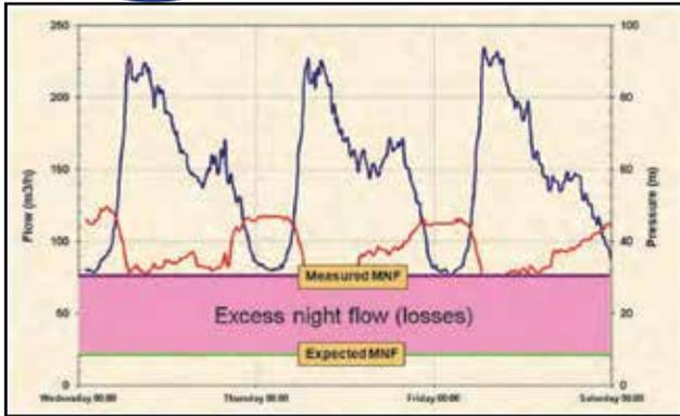
Figure 8: Example of a basic flow and pressure logging
