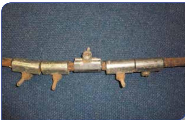
*Figure 12: A case where pipe replacement is clearly appropriate*
