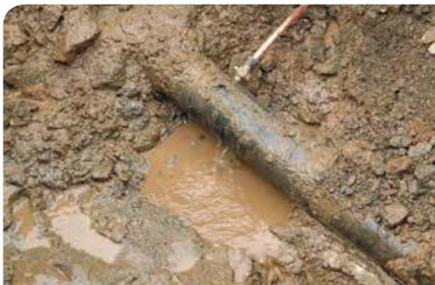
Figure 5: Underground leak running at low pressure (Ken Brothers)
