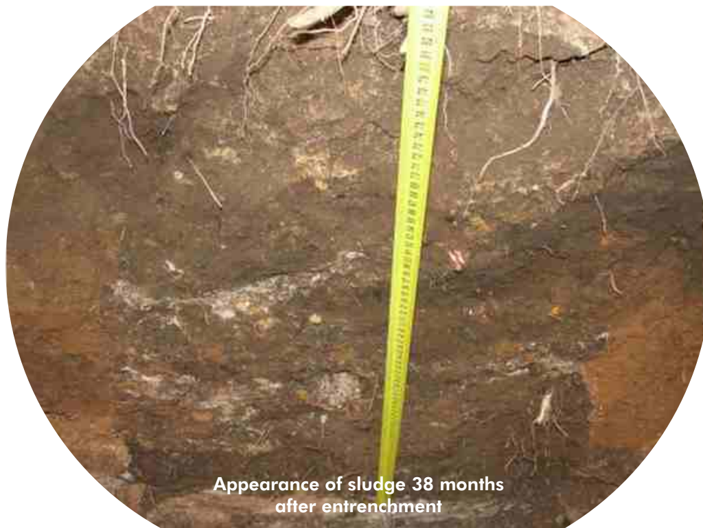
Fig.3. Entrenchment of sewerage sludge at the Sappi test site.
