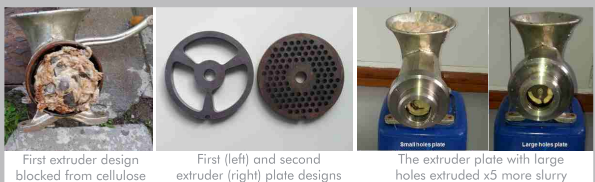
Fig.2. Extruder testing and modification for solar sanitising unit.
