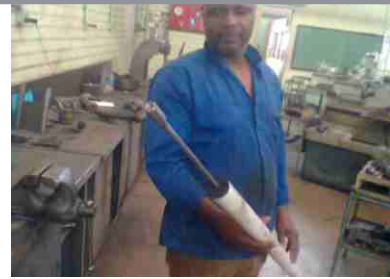
Suction sampling tool fabricated by team
