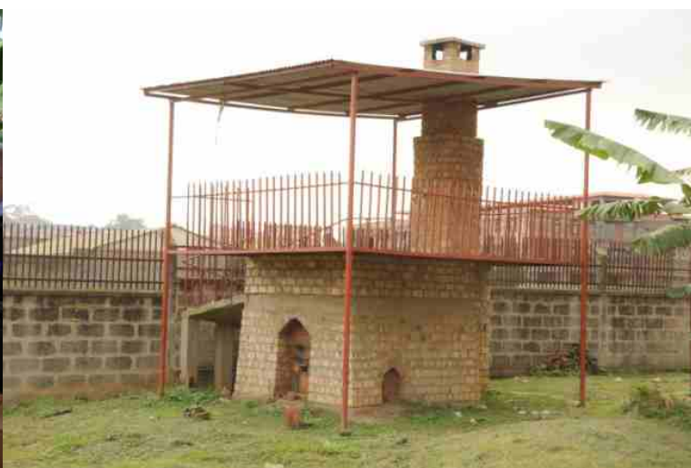
Fig.4 FaME pilot-scale kiln for brick production at Bugolobi wastewater treatment plant. Photo by Mortiz Gold, Sandec/EAWAG
