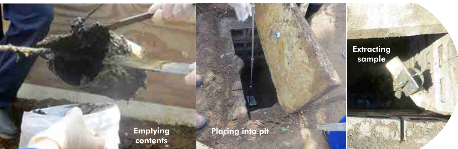
Fig.9. The “bucket” sampling tool for wetter sludge. The tool had a movable base and the length of the metal rod could be adjusted to different lengths.
