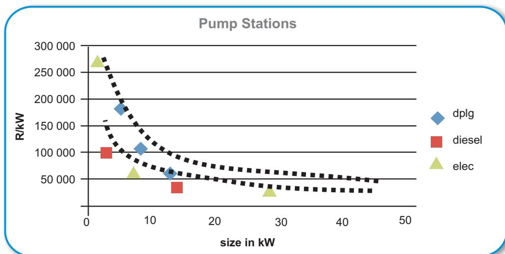
This chart demonstrates that the cost of constructing infrastructure is not necessarily linearly related to the size of the asset. In this example, the cost per installed kW of a pump-station decreases as the size of the facility increases. Small pumps serving small areas are considerably more expensive per unit of power than larger pumps.
