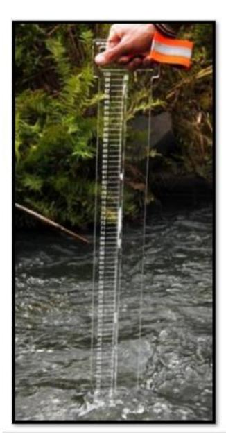
Measure water velocity and stream/river discharge
