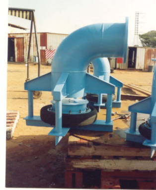
200 TO 400 DIAM DVs FOR FLOW CONTROL INTO IRRIGATION CANALS FOR MOZAMBIQUE
