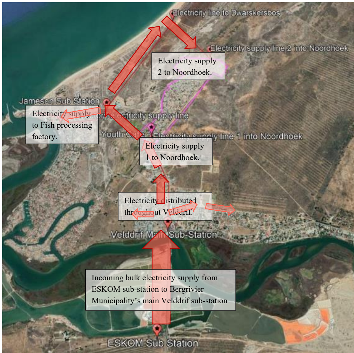
Figure 42 Electricity supply system of Velddrif, with a specific focus on the research area of Noordhoek, outlined in pink.
