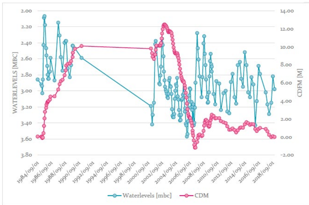
Figure 3.4: Time series graph of water levels for borehole G33323 with cumulative deviation from mean (CDM)
