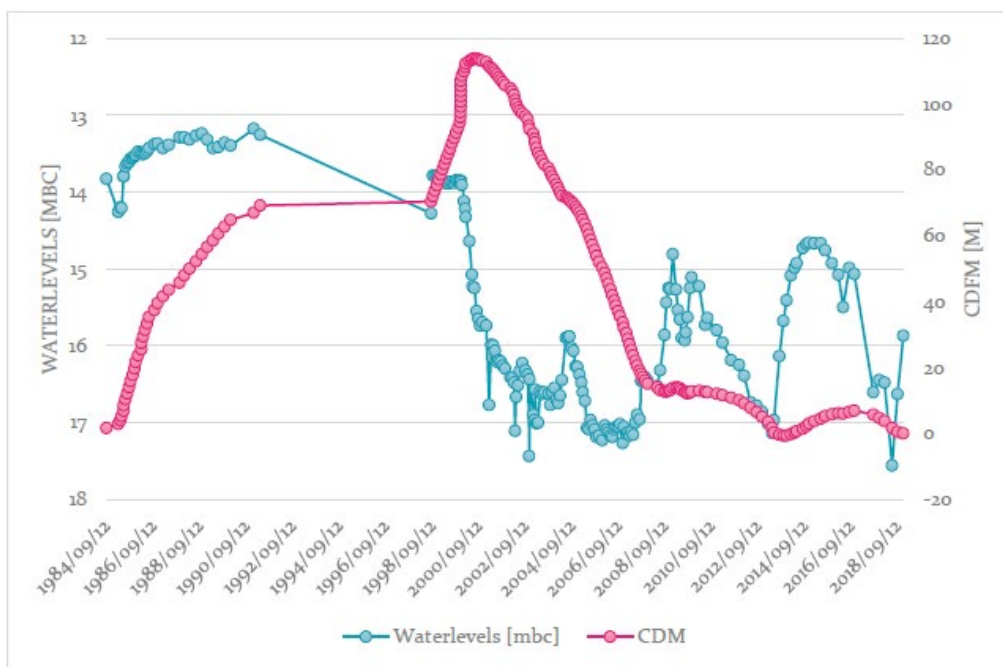
Figure 3.5: Time series graph of water levels for borehole G33327 with cumulative deviation from mean (CDM)
