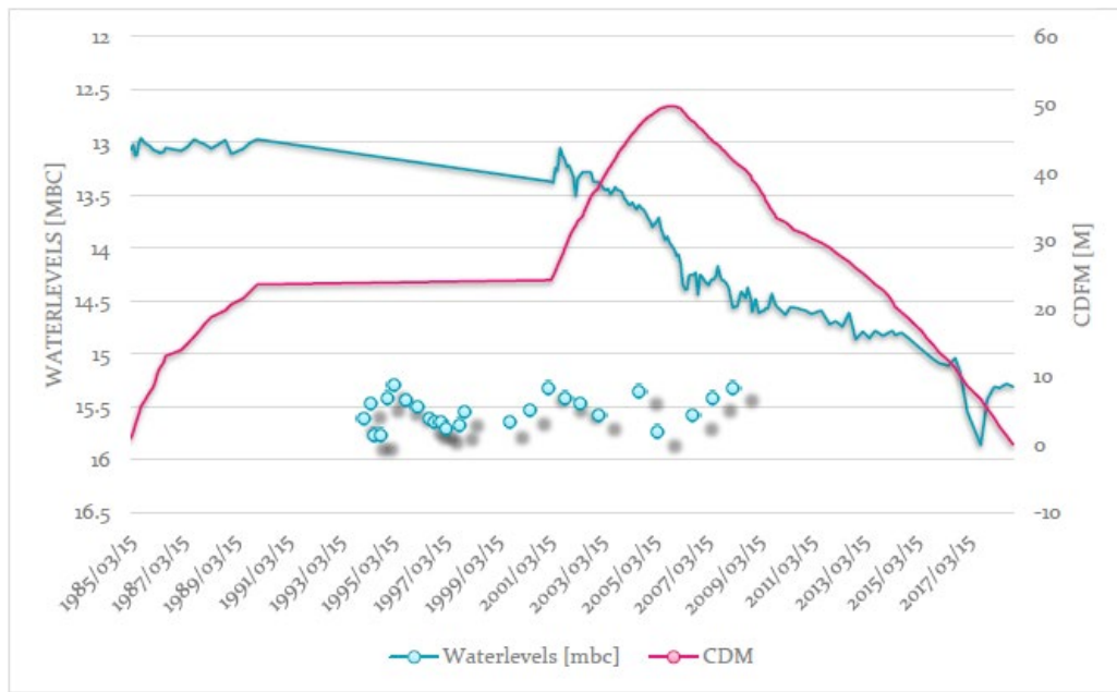
Figure 3.7: Time series graph of water levels for borehole G33317 with cumulative deviation from mean (CDM)
