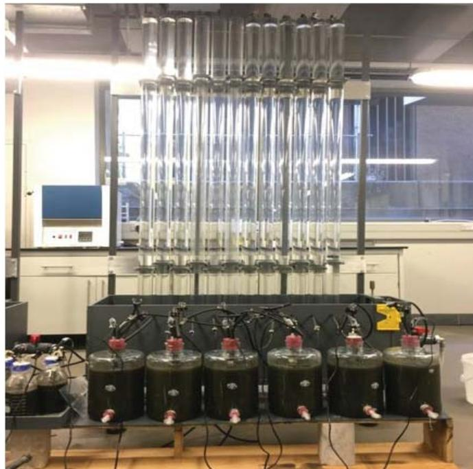
**Figure C 3. ABMP Test Setup in WQL at UCT**
