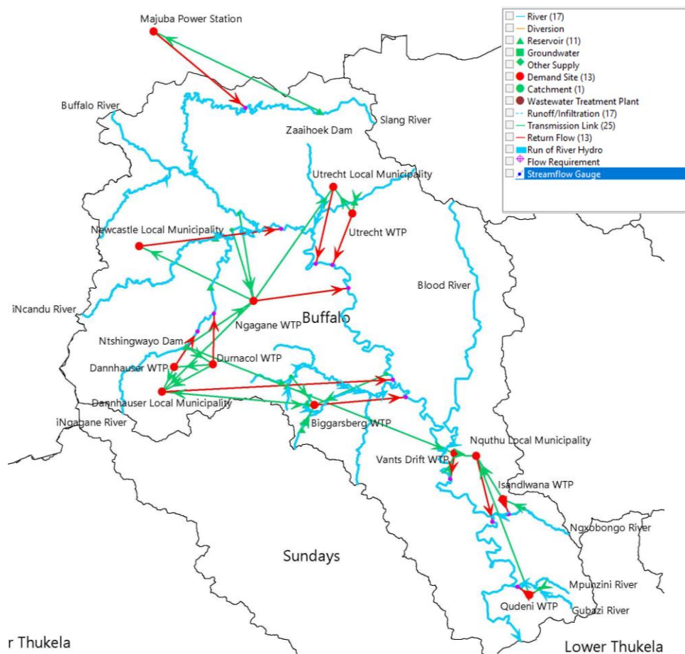
Figure 9.3 Schematic of the Buffalo River catchment with water demand sites and reservoirs.
