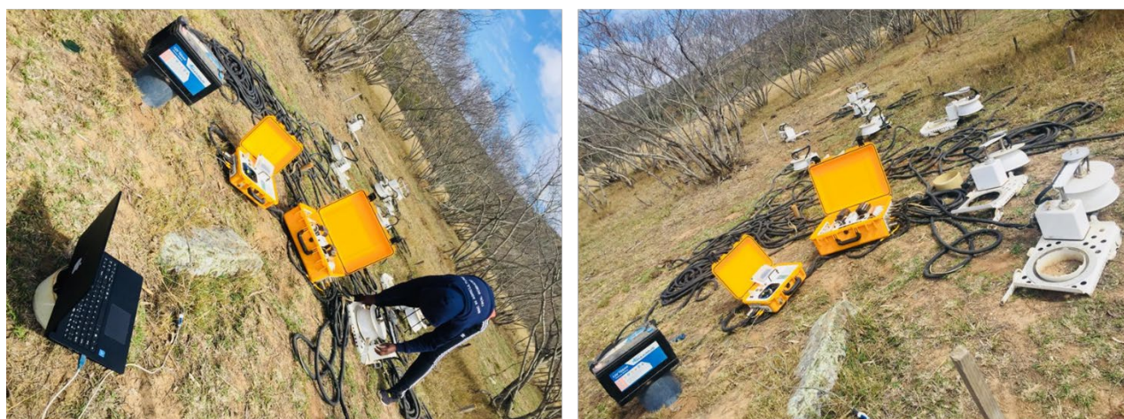
Figure 4.5: Setting up of the Li-Cor 8100 chambers for the measurement of CO 2 emission rates at Ncerha village in the Eastern Cape.
