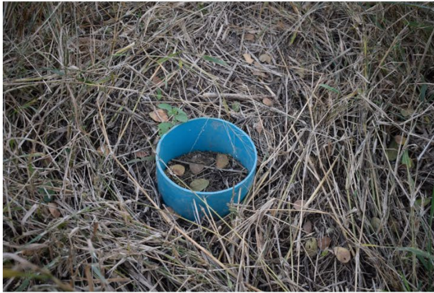
Figure 4.4: Chamber system used for CO 2 measurement in the Letaba catchment
