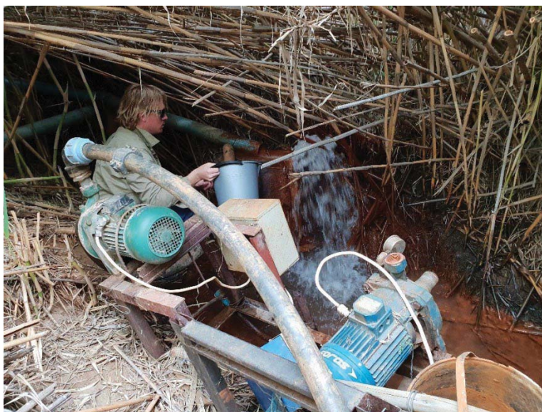
Figure 2-24 Groundwater sampling directly from spring outlet pipe.
