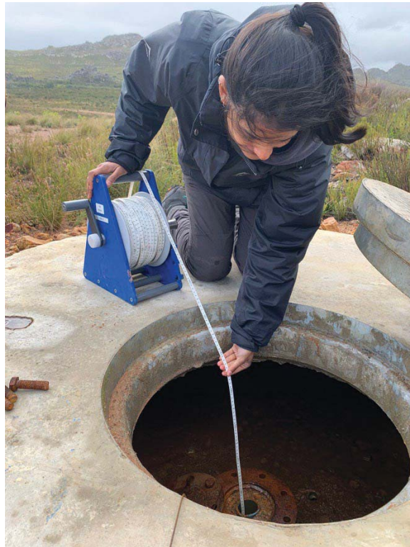
Figure 2-8 Dip meter used to measure groundwater levels.
