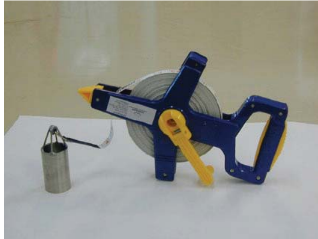
Figure 2-9 Plover used to measure groundwater levels (Sundaran et al., 2009).
