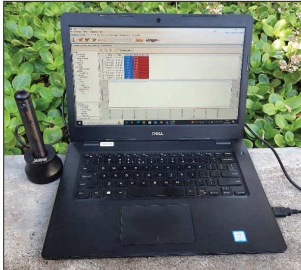
Figure 2-13 Manual water level datalogger download using logger docking station.
