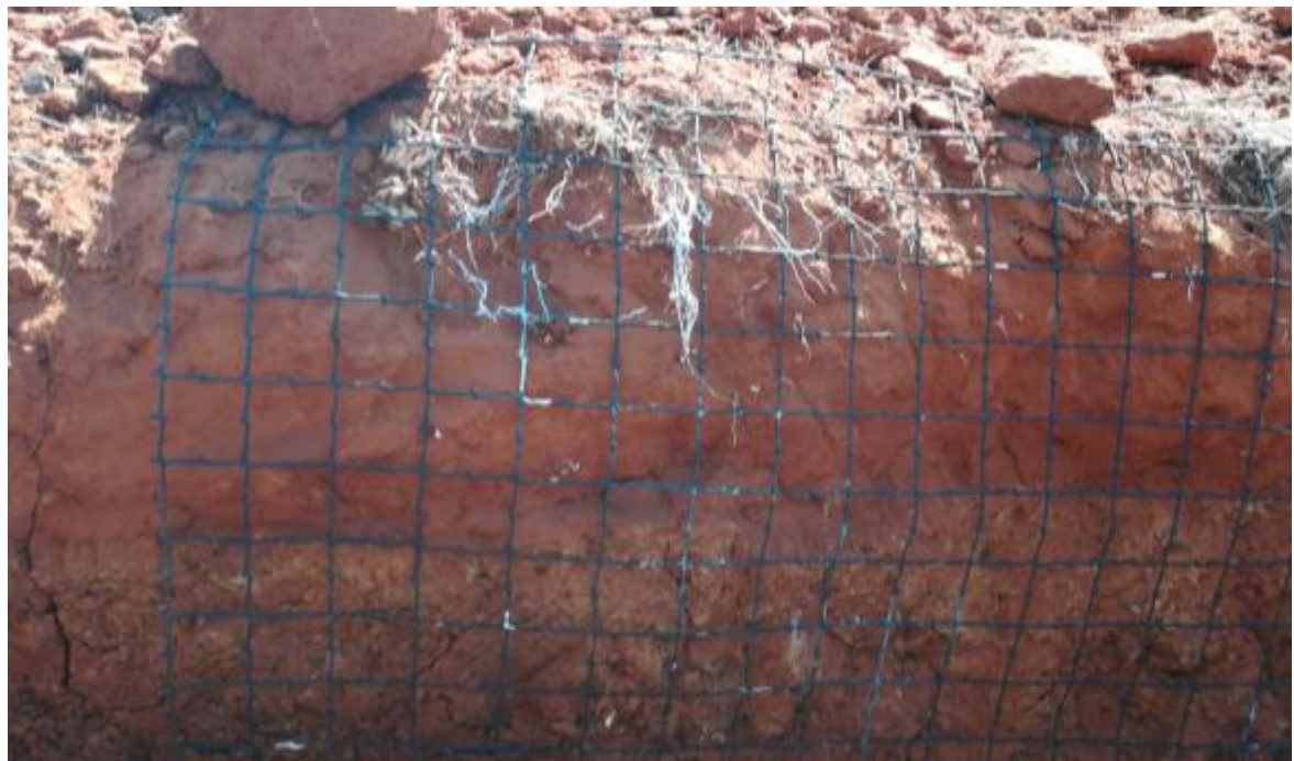
Photo 8: Vertical and lateral cracks in compacted layers in the cover at site D2-S5.
