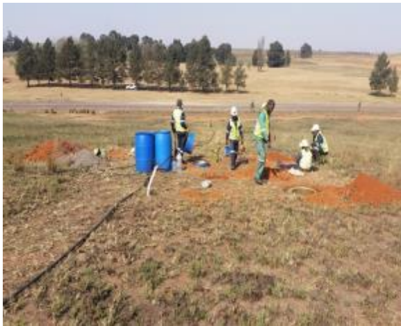
Photo 10: Setting up infiltrometer tests
