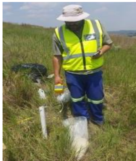
Photo 14: Measure oxygen concentrations
