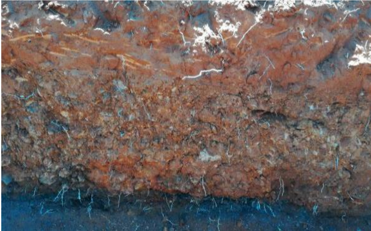
Photo 9: Fine cracks around concretions and weakly structured clayey layer.
