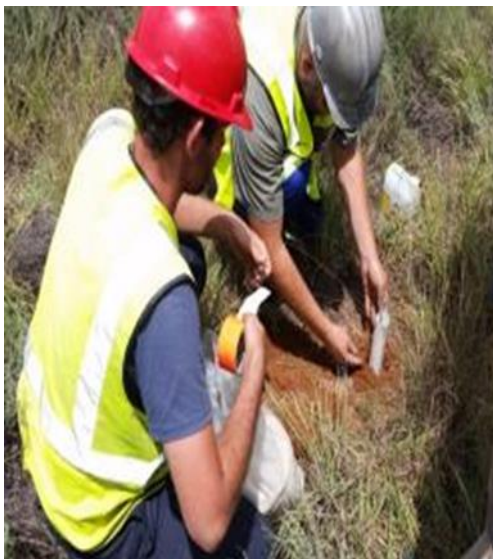
Photo 13: Install oxygen monitoring nest
