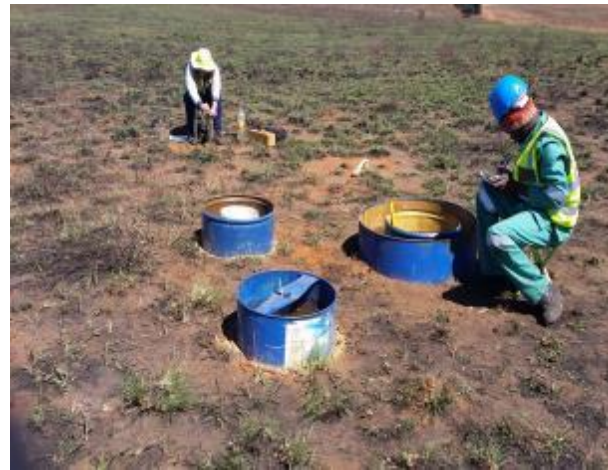
Photo 11: Conducting infiltrometer tests
