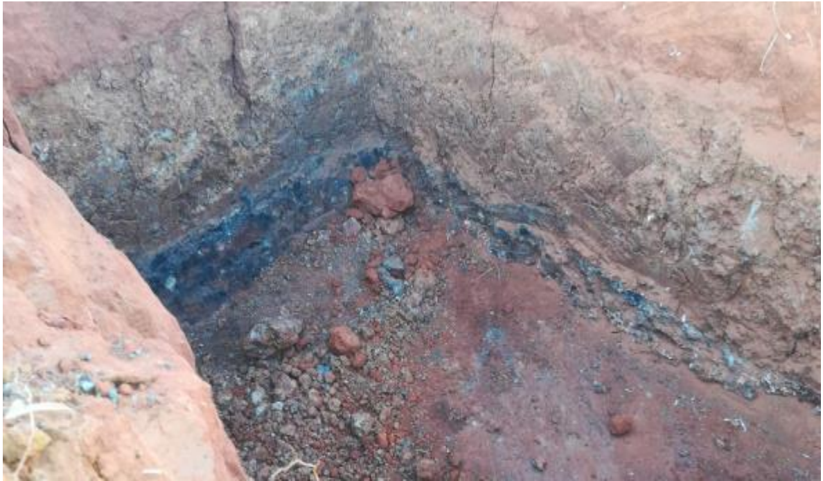
Photo 7: Vertical (tension) cracks in compacted layers in the cover at site D2-S4.
