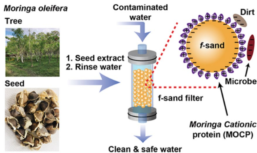
Figure 3.4: Moringa seed extract-functionalized sand filter (f-sand) to enhance colloidal and pathogen removal for potable water production with less to no residual organic matter production (Xiong et al., 2017).
