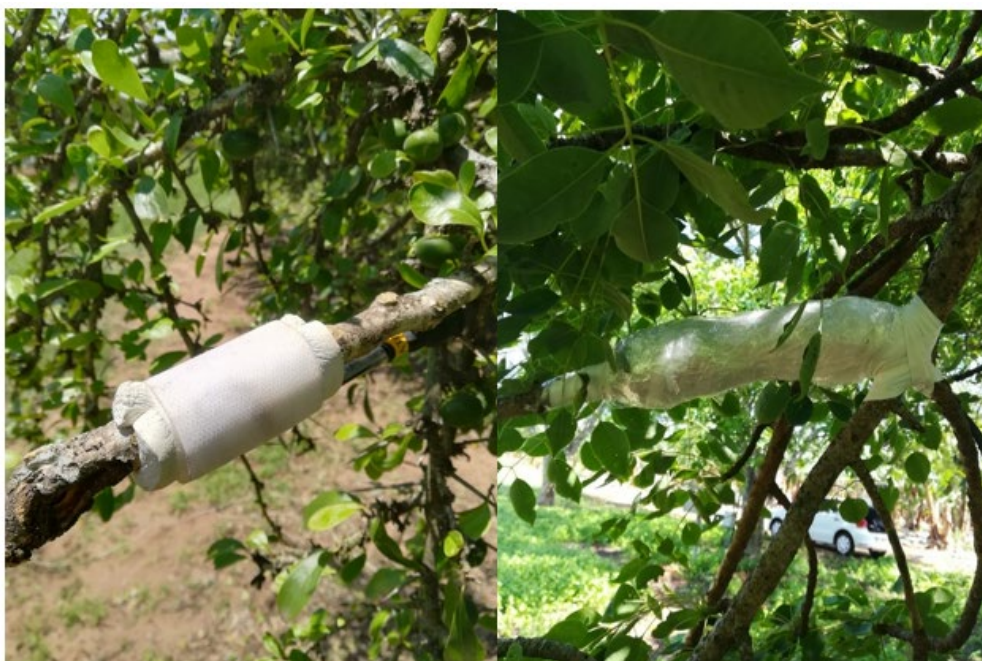
Fig. 4. 7. Sap flow gauges installed on the indigenous fruit tree branches
