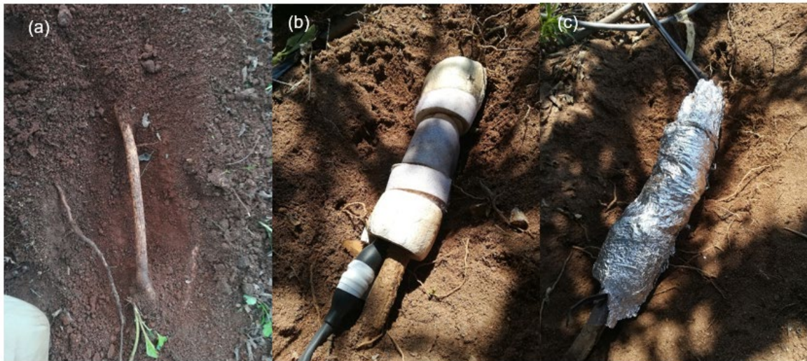
Fig. 4. 6. Installation procedure for the root sap flow sensors.
