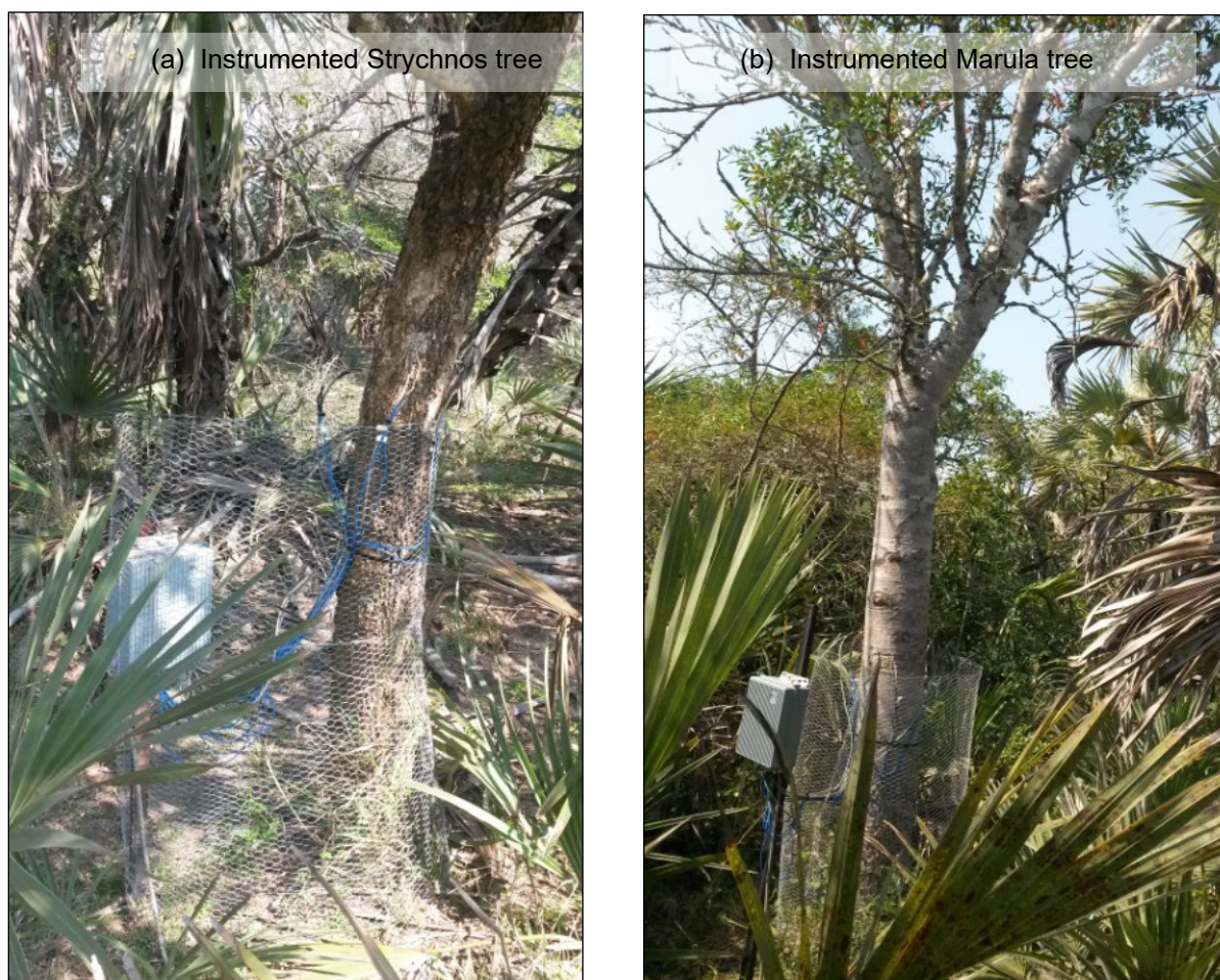
Fig. 3. 4. (a) Strychnos and (b) Marula instrumented with the heat ratio method sap flow probes at Bonamanzi Game Reserve.
