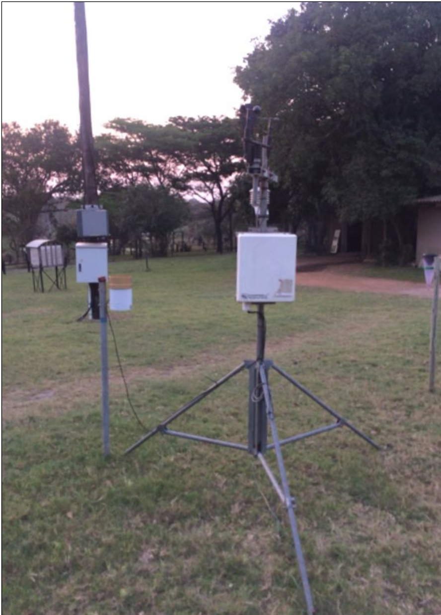
Fig. 3. 2. Automatic weather station measuring basic weather variables at Bonamanzi.
