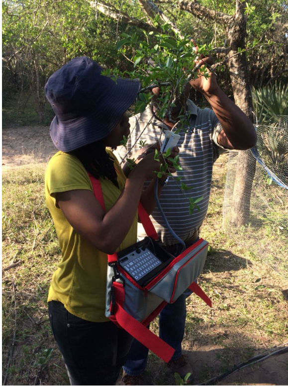
Fig. 3. 5. Measurement of the stomatal conductance of S. spinosa using the AP4 porometer.
