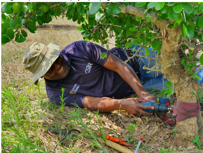
Fig. 5. 2. Installation of sap flow sensors on a Dovyalis tree at the ARC campus in Nelspruit
