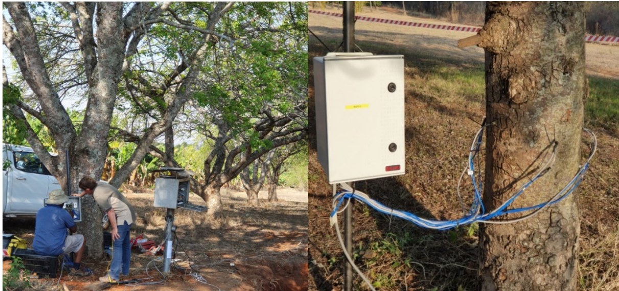
Fig. 4. 3. Heat ratio sap flow monitoring systems installed on the mature Marula trees at the ARC Burgershall research site
