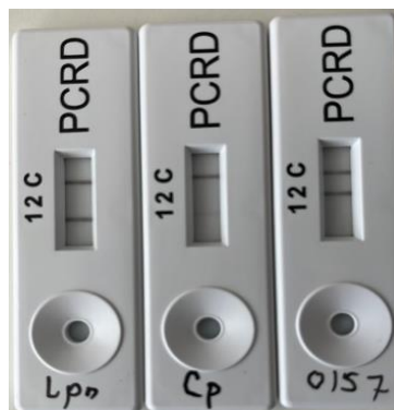
Figure 3-11. First test to discern if labelled amplicons are detected on PCR D device. Lpn = L. pneumophila ; Cp = C. perfringens ; 0157 = E. coli 0157:H7 . 10 ng input DNA and 37°C used as amplification temperature. Test line 1 must detect L. pneumophila and C. perfringens , while test line 2 detects E. coli 0157:H7 .
