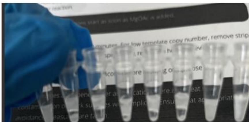
Figure 3-4: A test strip from the TwistAmp Basic kit, containing 8 PCR tubes with lyophilised RPA reagents. A rehydration buffer (provided in the kit) is added, plus the primers, water, template DNA, and magnesium acetate; the latter is added last, as it initiates the PCR reaction, which starts immediately.
