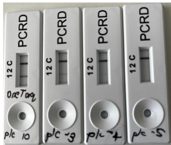
Figure 3-8: Lateral flow detection of C. perfringens amplicons generated by conventional PCR. Amplicons are labelled on both ends, on 5' end with DIG and on 3' end with Biotin. Only the amplicons generated with input DNA of Lane 2 (10 ng input DNA) as well as in Lane 5-7 in Figure 3-1 were used for LFA detection (Gel Lane 5: 0.01 ng aka 10 pg input DNA; Lane 6: 1 pg input DNA; Lane 7: 0.1 pg input DNA). 10fold serial dilutions was prepared from 10 n/ul of DNA, thus: plc^{-3} = input DNA in PCR was 10 ng x 10^{-3} dilution/0.1 ng DNA/10 picogram input DNA.
