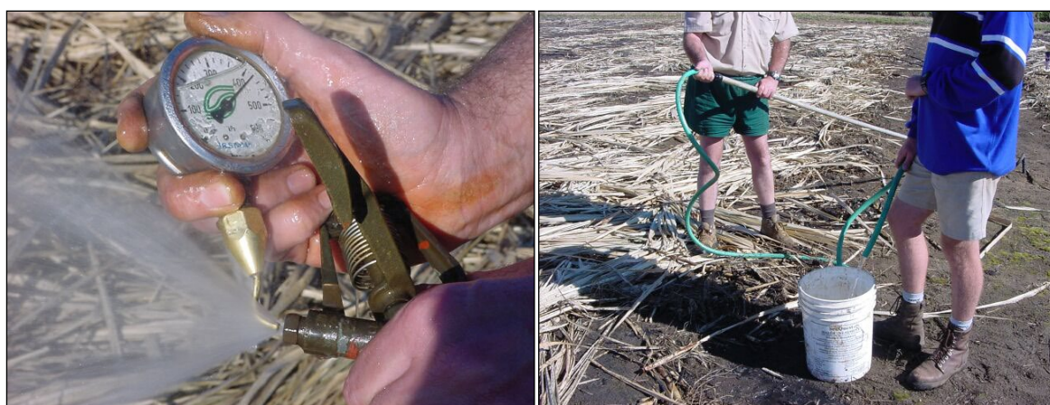
Figure 4: Pressure and flow rate measurement (adapted from Koegelenberg and Breedts, 2003)
