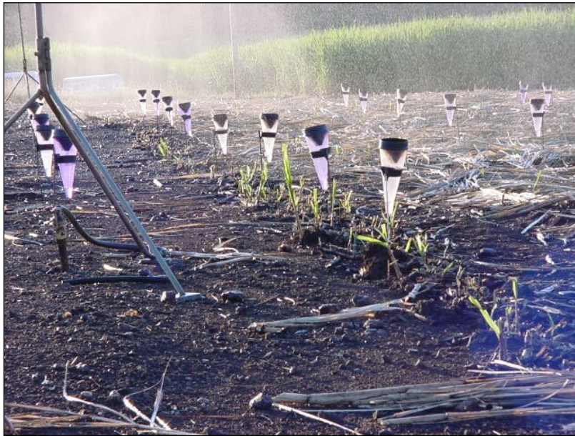
Figure 5: Rain gauge set-up to measure the distribution of water under a dragline sprinkler (adapted from Koegelenberg and Breedts, 2003).
