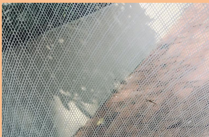
Plastic mesh for covering perforations around the borehole casing
