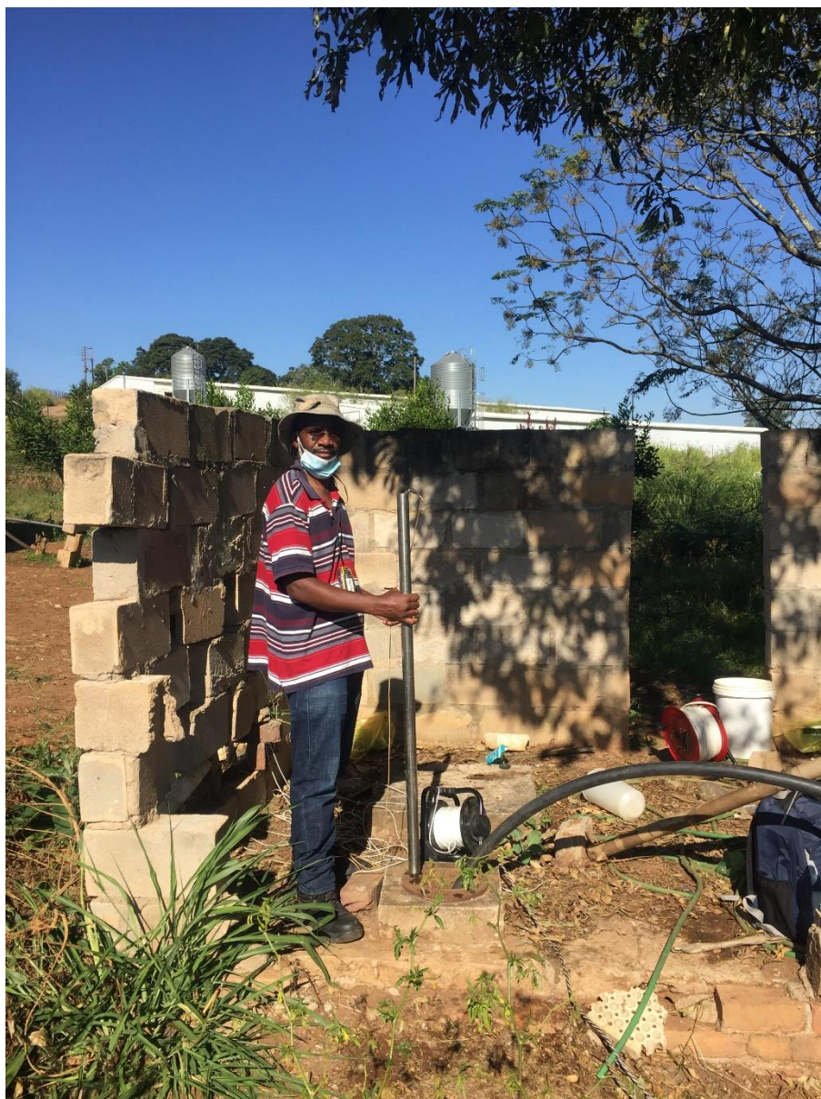
Figure A2: Groundwater sampling using a bailer and water level measurement at one of the unequipped boreholes in White River (White River – BH3) in 2021.
