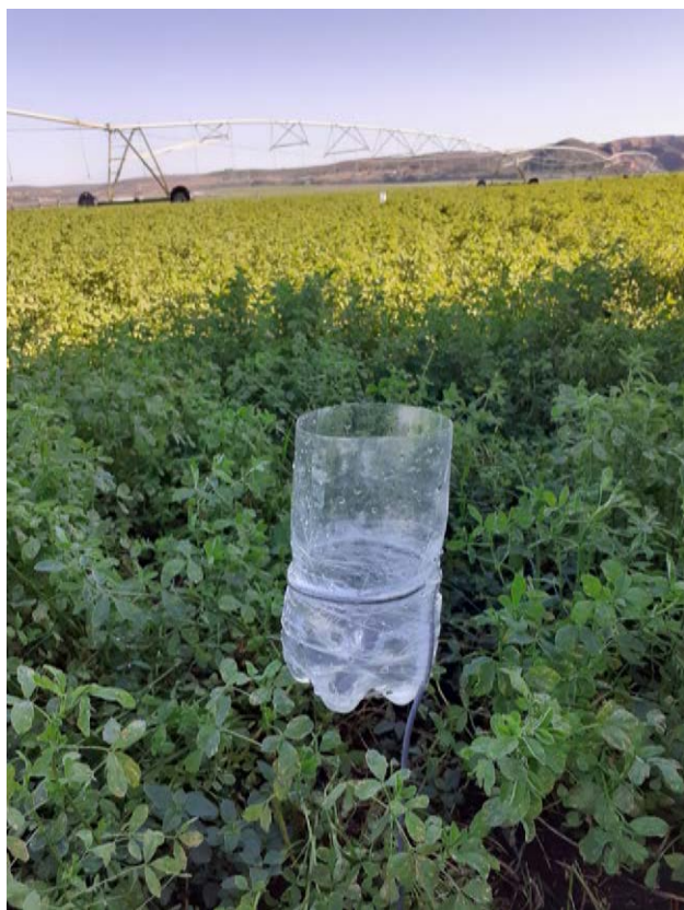
A 'catch can test' in action, to test the irrigation efficiency of pivots. Water droplets are captured to calculate efficiency measures (calibration, system and scheduling).
