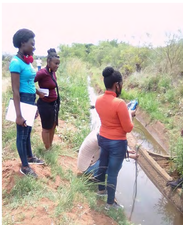
Figure 5.10: Flow measurement at offtake structure in Mandiwana irrigation scheme
