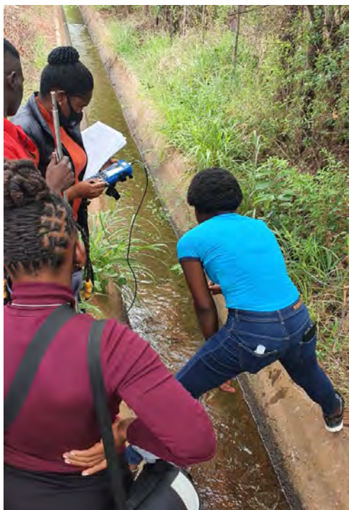
Figure 5.9: Flow measurement at Parshall flume in Raliphaswa irrigation scheme
