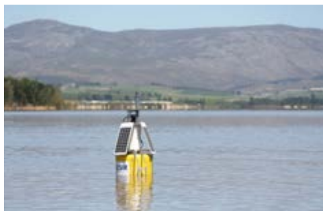
Gizmo, Africa's only hyperspectral radiometric buoy, deployed in Theewaterskloof Dam.
