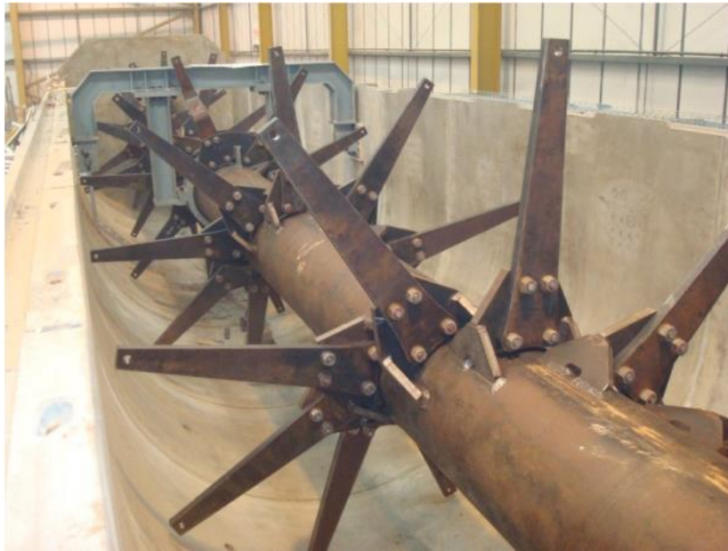
Figure 3.2. The internal mixing tine-bearing shaft of the standard HotRot, designed for control of this in-vessel composting process.
