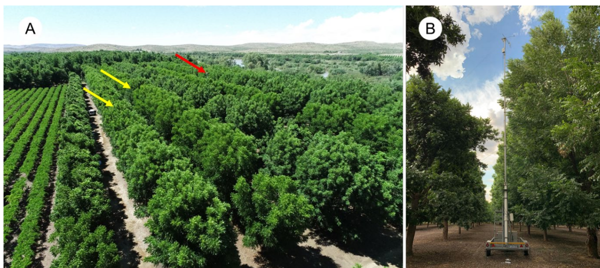
Figure 3.15 A) Positioning of the Eddy Covariance system in the Groblershoop orchard installed in September 2020. The red arrow indicates the positioning of the tower, whilst the yellow arrows indicate the locations of the transpiration measurements. B) The Eddy covariance tower within the work row.
