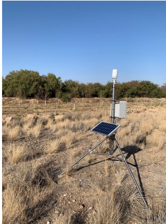
Figure 3.9 The automatic weather station installed within 250 m of the study orchard on the farm close to Groblershoop
