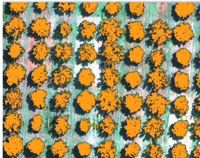
Figure 3.28 Individual canopy polygons created using threshold value of simple ratio index (SRI)
