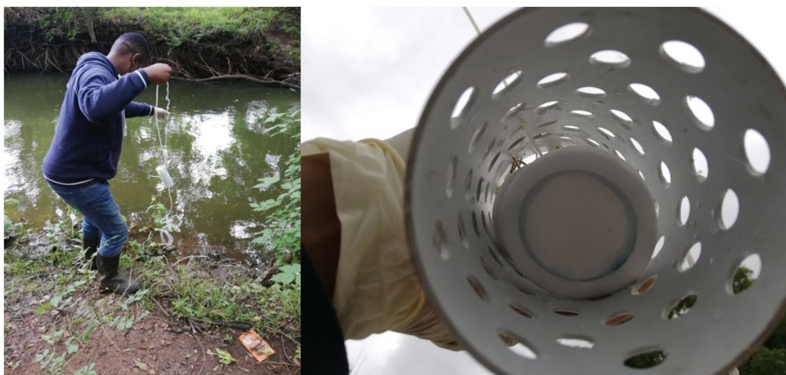
Figure 5.2. Field deployment of POCIS passive samplers (left), POCIS placed inside a cage (right) (Photograph: T. Letseka)
