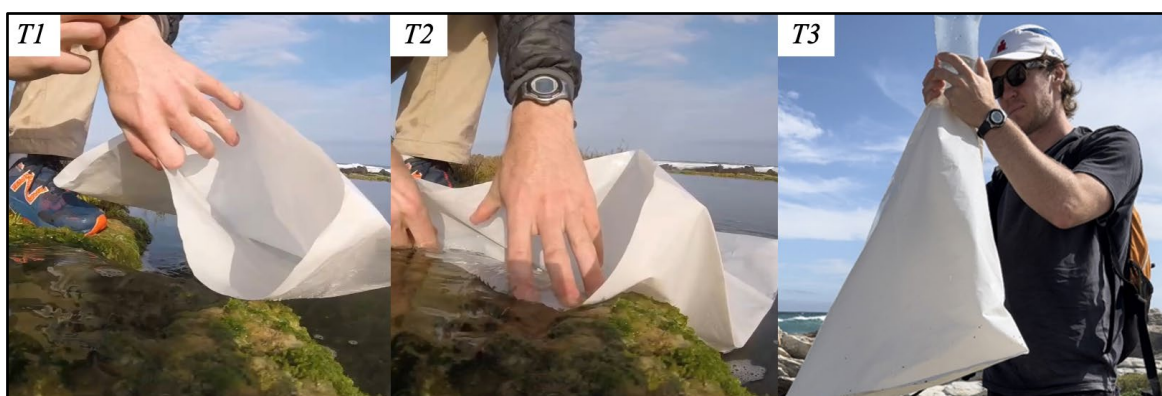
Figure 10. The Capture Cup method. Water is funnelled into a plastic bag for a set amount of time (T2) and then measured in a volumetric beaker to calculate the flowrate (T3).
