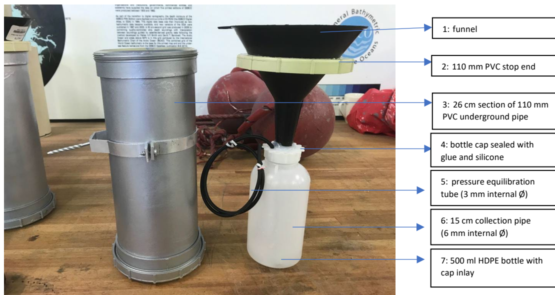
Figure 46. Dip-in precipitation totaliser sample unit (right) that was placed inside the PVC pipe containing unit (left).
