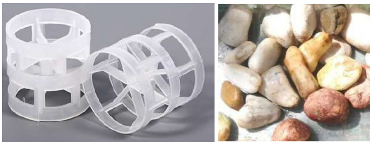
Figure 3.5. Pebbles and polypropylene pall rigs used as packing material during the tests of the urine evaporator
