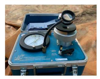
Figure 28. A Scholander pressure chamber used for determining leaf water potential.
