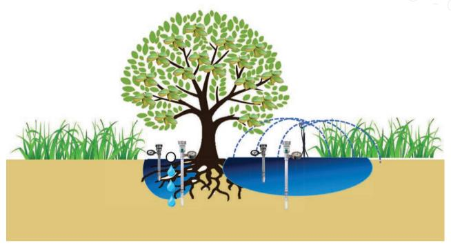
Figure 25. Placement of tensiometers within and below the root zone to trigger irrigation events and to monitor the depth of irrigation. The shallow tensiometer indicates when irrigation should start and the deep indicates when irrigation should stop.
