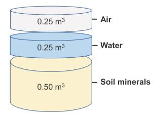
Figure 11. Soil constituents in a known volume of soil. All the components total 100%. Since volumetric water content (VWC) equals the volume of water divided by the total volume of soil, the VWC in this example would be 25%.
