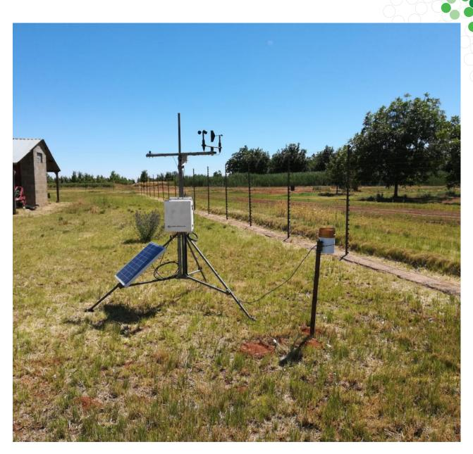
Figure 30. An automatic weather station installed over a short grass reference surface.
