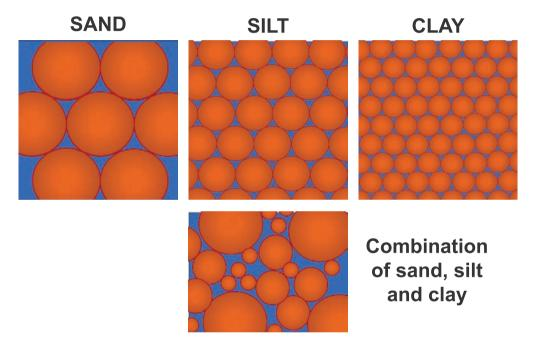
Figure 13. Variation in particle sizes and how this impacts pore space in a soil. Also note the varying surface area around different sized particles – the smaller the particles the greater the overall surface area.
