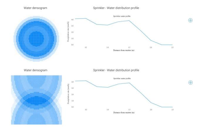
Figure 5. Examples of water densograms from sprinklers and water distribution profiles from a sprinkler. Data was generated from Netafim's NetSpeX<sup>™</sup> website.
