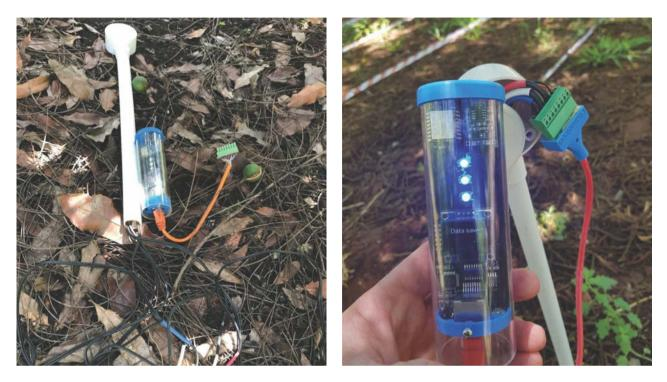
Figure 26 Chameleon soil water sensors and wifi reader for determining soil matric potential at three different depths.
