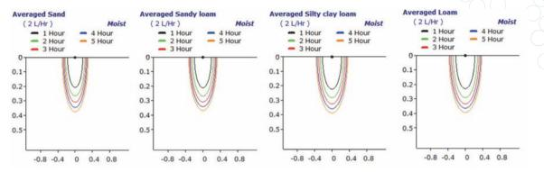
Figure **7**. Wetting patterns in different textured soils from a 2 L h<sup>-1</sup> dripper run for 5 hours
