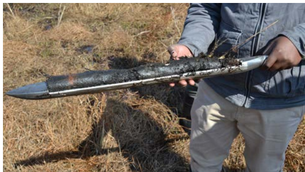
Peat is extracted from the Wterkloofspruit peatland system using a peat auger.
