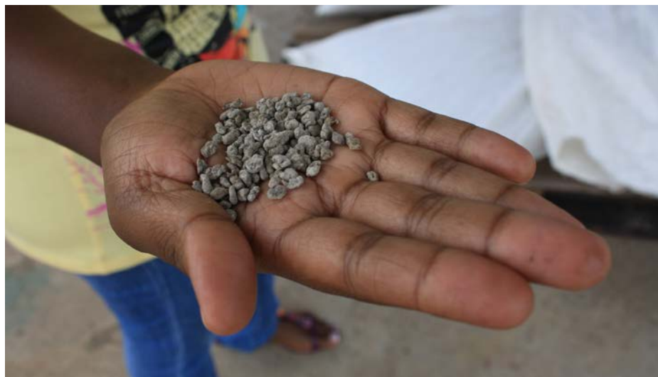
Treated and dried sludge pellets, which can be sold as fertilizer.
