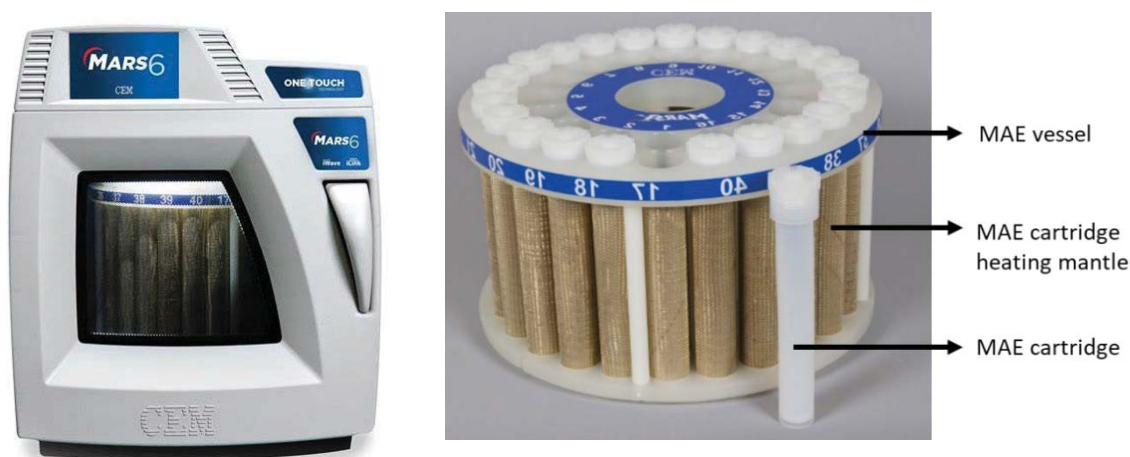
Figure 2-6: Illustration of the microwave-assisted extractor (MAE) and the setup of the MAE vessel for sample processing
