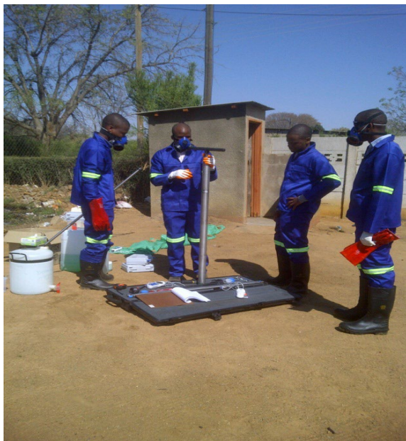
FIGURE 2-2: PREPARATION OF THE SAMPLER FOR SAMPLING (A) AND THE SAMPLING PROCESS THROUGH THE SQUAT HOLE (B)
