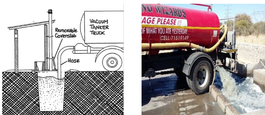
FIGURE 3-6: METHOD OF PIT EMPTYING IN BOTSWANA (LEFT) AND A PRIVATE VACUUM TRACK DISCHARGING AT THE GABORONE WASTEWATER TREATMENT PLANT DISCHARGE BAY (RIGHT)
